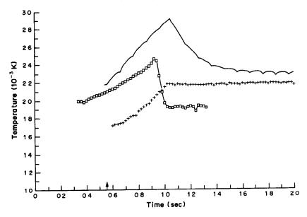
Fig 4 The surface and vapour temperature profiles of SP-9 modified tube II during wall atomization at 2273 K Symbols as for Fig 2
