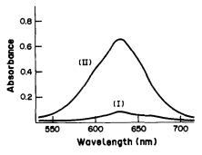
Fig. 1. Absorption spectra: (I), reagent blank; (II),  $4.1 \times 10^{-6} M$  Ge (1.2  $\mu$ g). Malachite Green,  $5.0 \times 10^{-4} M$ ; mandelic acid,  $1.5 \times 10^{-3} M$ ; pH, 3.0; reference, chlorobenzene.
