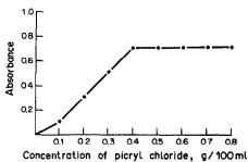
Fig. 2. Effect of picryl chloride concentration on the absorbance of the product from imipramine HCl (5  $\mu$ g/ml).
