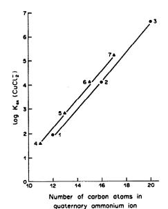
Fig. 6. Relation between log K<sub>ex</sub>(CuCl<sub>2</sub><sup>-</sup>) and number of carbon atoms in the quaternary ammonium ion. Tetra-alkylammonium cations (♠): 1, TPA<sup>+</sup>; 2, TBA<sup>+</sup>; 3, TAA<sup>+</sup>. Alkyltrimethylammonium cations (♠): 4, OTMA<sup>+</sup>; 5, DTMA<sup>+</sup>; 6, DDTMA<sup>+</sup>; 7, TDTMA<sup>+</sup>.
