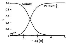
Fig. 6. Distribution of Pd(II) species in the Pd(II)-NMP system as a function of pH.  $C_L = 5 \times 10^{-5} M$ ,  $C_M = 1 \times 10^{-5} M$ .
