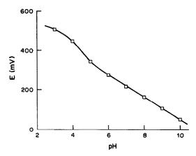
Fig. 5. Potentiometric pH response of a typical TDDA-doped hydroxylated asymmetric membrane. The pH was adjusted by the addition of sodium hydroxide to a buffer containing 11.4mM boric acid, 6.7mM citric acid, and 10.0mM NaH<sub>2</sub>PO<sub>4</sub>, and monitored with a glass membrane electrode.
