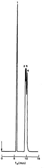
Fig. 5. Chromatogram of model mixture of cresols and phenol: (1) o-cresol, (2) m-cresol, (3) p-cresol, (4) phenol. Column Silasorb 600, 6  $\mu$ m, 120  $\times$  2 mm; mobile phase 70% v/v methylene chloride in n-hexane; 25°C; spectrophotometric detector (270 nm).
