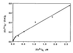
Fig. 9. Plot of  $[Cu^{2+}]_2/[CuL]_2$  vs.  $[Cu^{2+}]_2$  for the Willamette River water sample.
