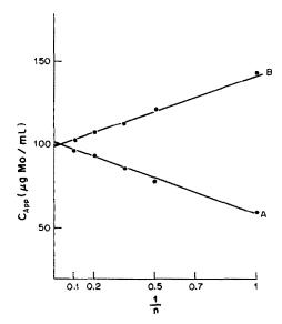
Fig. 9. Determination of molybdenum in the presence of calcium in the air-acetylene flame. Test sample: 100  $\mu$ g Mo/ml and 3 mg Ca/ml. Curve A: without buffer interferent;  $c_{App_{\infty}} = 101 \ \mu$ g/ml. Curve B: buffer interferent 5 mg V/ml;  $c_{App_{\infty}} = 99 \ \mu$ g/ml.
