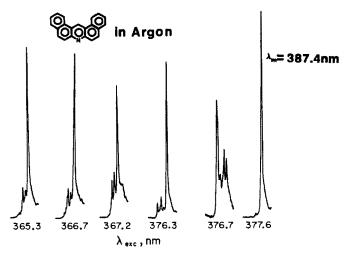
Fig. 1. Fluorescence spectra of dibenz[a, j]acridine in solid argon at 15 K as a function of excitation wavelength (indicated at bottom of each spectrum). For each spectrum, the total wavelength range scanned was 5 nm (385-390 nm).
