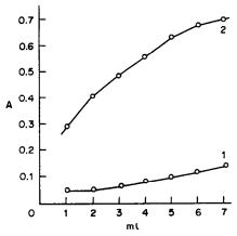
Fig. 4. Dependence of reaction rate on amount of acetic acid. (1) Uncatalysed reaction; (2) catalysed reaction; 1.0  $\mu$ g of Fe(III) per 25 ml.
