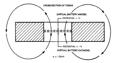
Fig. 6. Potential method for cell analysis. A very thin disc is pictured, centered in the toroid, with the upper surface of the disc at a potential of +1/2 and the lower surface of the disc at a potential of -1/2. The total current flowing from the anode to the cathode (through a solution with conductivity 1 S/cm) in this imaginary battery is numerically equal to the cell constant.
