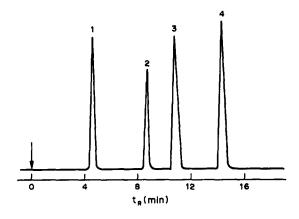
Fig. 2. Chromatogram of model mixture of nitrophenols and phenol: (1) o-Nitrophenol. (2) m-nitrophenol, (3) phenol, (4) p-nitrophenol. Column Silasorb 600, 10  $\mu$ m, 200  $\times$  6 mm; mobile phase 1% v/v propan-2-ol and 6% v/v diethyl ether in n-hexane; 25°C; spectrophotometric detector (270 nm).
