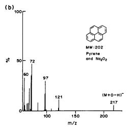
Fig. 5. Negative-ion LMS of (a) Na<sub>2</sub>O<sub>2</sub>, (b) pyrene mixed with Na<sub>2</sub>O<sub>2</sub>.
