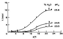
Fig. 5. Response time for establishment of pH equilibrium (±0.003) for a glass electrode in different DMSO/water mixtures (Radiometer G 202B and Ag/AgCl electrodes).
