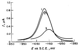
Fig. 1. Differential pulse polarograms for the reduction of iodate  $(9.8 \times 10^{-6} M)$ : 1, in 5M NaClO<sub>4</sub>; 2, in 4M  $NaClO_4 + 1M$  NaCl; 3, in 4M NaClO<sub>4</sub> + 1M NaSCN.
