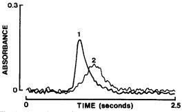
Fig. 4. Absorption profiles for  $25 \mu g/l$ . tin in modifier A: 1, pyrolytically coated tube and pyrolytic graphite platform; 2, tube and platform as for 1 but coated with tungsten.
