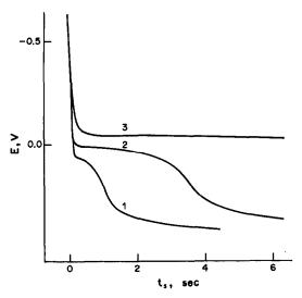
Fig. 2. Potentiometric stripping curves obtained for 3  $\mu$ g/ml Ni(II) in 1% ammonia solution deaerated for 1 (1), 4 (2) and 10 (3) min:  $t_d = 3.0$  min,  $t_r = 1.0$  min. Reduction potential -1.15 V vs. SCE.
