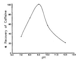
Fig. 4. Influence of pH on extraction of caffeine from mixtures with theophylline. Whatman No. 1 filter paper treated with 3 μ1 of 1M KI. Excitation and emission wavelengths are 275 and 440 nm, respectively.
