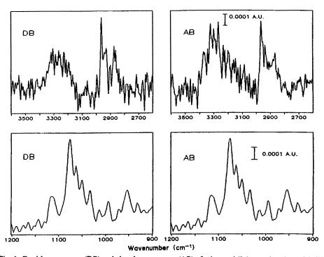
Fig. 6. Dual-beam spectra (DB) and absorbance spectra (AB) of n-butanol (0.1 monolayer) on nickel(100) at 150 K.
