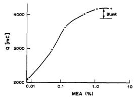
Fig. 5. Efficiency of carbon dioxide absorption at various concentrations of MEA in 2-propanol + water (98 + 2).
