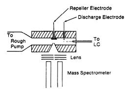
Fig. 5. Schematic diagram of Finnigan-MAT TSP ion source showing location of discharge and repeller electrodes.
