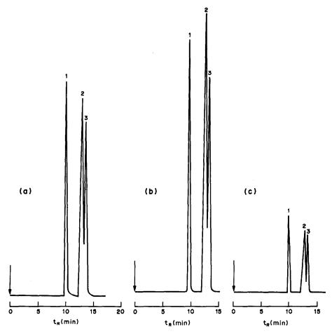
Fig. 6. Chromatograms of a model mixture of cresols and phenol (1) o-cresol, (2) m- and p-cresols, (3) phenol. Column Silasorb 600, 6 μm, 120 × 2 mm; mobile phase 1% v/v propan-2-ol in n-hexane; 25°C; spectrophotometric detector: (a) 210, (b) 218, (c) 270 nm.
