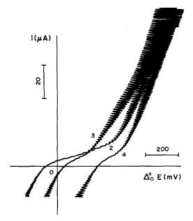
Fig. 5. Polarogram of the HTTA-La-TOPO adduct. Aqueous phase: 0.2M NaOAc, 0.4mM La, pH 6.0 ± 0.1. DCE phase: 0.01M THA TPB; (1) 5mM HTTA, (2) 2.8mM TOPO, (3) 5mM HTTA, 2.8mM TOPO.
