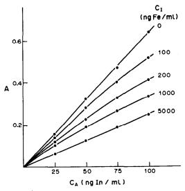
Fig. 5. Effect of iron (as ferric chloride) on the calibration curve for indium in a graphite tube at 2000°.
