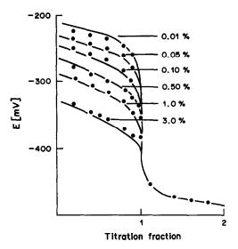
Fig. 4. Effect of MEA concentration on the titration curves of MEA + CO<sub>2</sub> reaction product in 2-propanol + water (98 + 2). The amount of carbon dioxide is ca. 0.05 mmole. Points—experimental; solid lines—calculated for MEAH<sup>+</sup> in the presence of an excess of MEA.
