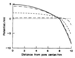
Fig. 2. As for Fig. 1, except that there is a surface charge density of  $-1.0 \times 10^{-12}$  mole/cm<sup>2</sup> on the edge of the pore. The salt is equally soluble in the stationary phase and the mobile phase. The concentration of added salt (that is, not including the counter-ion to the fixed charges) is  $0M \longrightarrow 10^{-3}M \longrightarrow 10^{-3}M \longrightarrow 10^{-1}M \longrightarrow 10^{$
