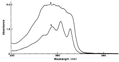
Fig. 2. The effect of concentration on the absorption spectrum of BAC. (a) Below the cmc; (b) above the cmc.
