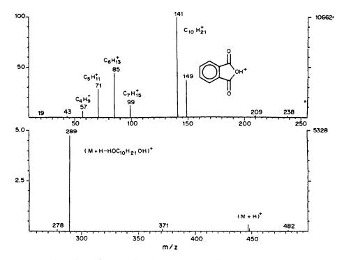
Fig. 4. MS/MS daughters of m/z 447 for unknown component D; collision energy 20 eV, with argon.
