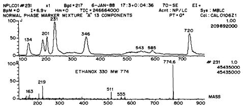
Fig. 7. Moving belt LC/MS (70 eV EI) of mixture of polymer additives. Total ion current (upper) with mass spectrum of major component (lower).
