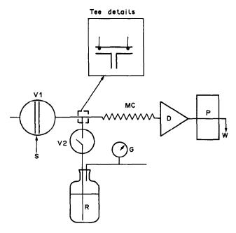
Fig. 4. A pulsed reagent-introduction system in ACCAS. Inset shows platinum resistance probes located in the tee. V1: six-port rotary loop injector; V2: on/off valve; G: pressure gauge; reagent bottle is pneumatically pressurized; other symbols as in Fig. 1.
