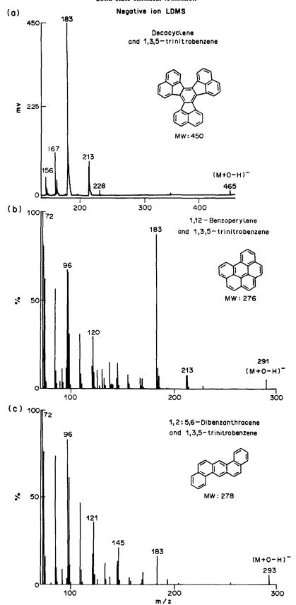
Fig. 2. Negative-ion LMS of (a) decacyclene, (b) 1,12-benzoperylene, (c) 1,2,5,6-dibenzanthracene, mixed with trinitrobenzene.
