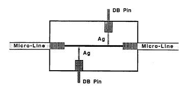
Fig. 3. Illustration of the biamperometric flow cell.
