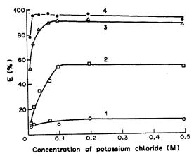
Fig. 4. Effect of aqueous phase concentration of potassium chloride on extraction of copper with alkyltrimethylammonium ions. Initial concentration of alkyltrimethylammonium ion in the aqueous phase is  $1 \times 10^{-3} M$ . 1, OTMA<sup>+</sup>; 2, DTMA<sup>+</sup>; 2, DDTMA<sup>+</sup>; 4, TDTMA<sup>+</sup>.
