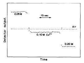
Fig. 10. ACCAS output at 1800 samples/hr; the sample was changed from 0.05 to 0.10 to 0.20 M Cu<sup>2+</sup> during the run.
