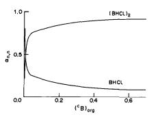
Fig. 2. The fraction of monomer (BHCl) and dimer (BHCl)<sub>2</sub> in the organic phase as a function of total amine concentration.
