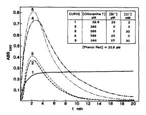
Fig. 1. Effect of CT and chloride concentrations on the kinetics of colour production and decay (measured at 590 nm).
