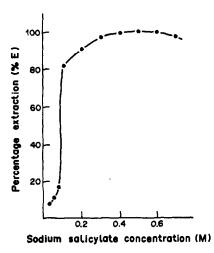
Fig. 2. Effect of sodium salicylate concentration for extraction of zinc.
