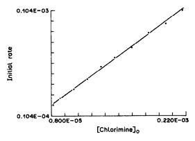
Fig. 7. Plot of the initial reaction rate vs. the initial concentration of chlorimine for the reaction of a series of chlorimine solutions  $(1.1 \times 10^{-5}-2.2 \times 10^{-4}M)$  with  $9.54 \times 10^{-3}M$  phenol at pH 9.71. Slope = 0.446. Standard error of the estimate =  $6.6 \times 10^{-6}$ . Variance of the slope =  $9.8 \times 10^{-4}$ .
