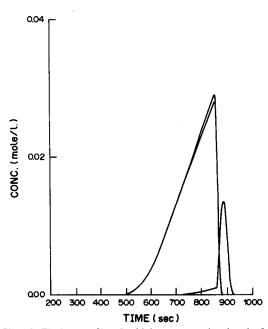
Fig. 12. Elution profile of a high concentration band of a binary mixture eluted with a binary solvent. Concentration of strong solvent: 0.1 M. Ratios of first Langmuir isotherm coefficients: solute 2/solute 1, 1.2; strong solvent/solute 1,
