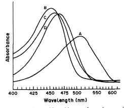
Fig. 1. Spectra of murexide and its complexes: A, murexide; B, Ni<sup>2+</sup>-murexide; C, Co<sup>2+</sup>-murexide; D, Cu<sup>2+</sup>-murexide.
