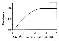
Fig. 2. Effect of picrate concentration on formation and extraction of the complex. Absorbance measured at 600 nm against a reagent blank;  $10~\mu g$  of iron; 1~ml of 10% hydroxylammonium chloride solution; 1~ml of buffer, 10~ml of  $10^{-3}M$  TPTZ, aqueous phase volume 100~ml, DCE 10~ml.
