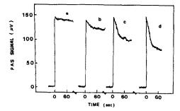
Fig. 3. Changes in photoacoustic signal amplitudes when a 460-nm laser beam was incident on Hg(II) dithizonate solutions in (a) benzene, (b) CHCl<sub>3</sub>, (c) CH<sub>2</sub>Cl<sub>2</sub> and (d) CCl<sub>4</sub>.
