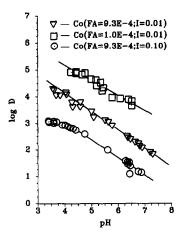
Fig. 3. The variation of the distribution coefficient (D) of Co(II) in the presence of fulvic acid, as a function of pH and ionic strength.
