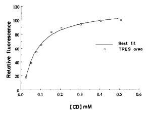
Fig. 4. TRES area vs. γ-CD concentration for pyrene-γ-CD complex in the presence of benzyl alcohol, with nonlinear least-squares curve-fitting to equation (3).
