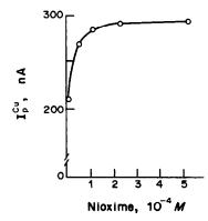
Fig. 4. Dependence of DP-AV peak current for  $5\times 10^{-8}M$  Cu in 0.1M ammonia buffer on nioxime concentration.  $E_{\rm acc}=-0.2~{\rm V},~t_{\rm acc}=60~{\rm sec.}$
