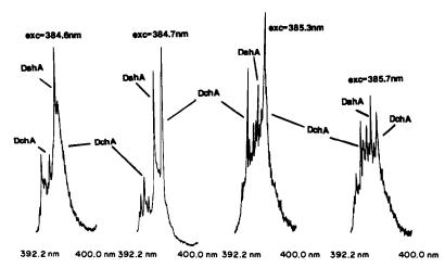
Fig. 5. Fluorescence spectra of four-component dibenzacridine mixture in solid n-octane (at 15 K) at various excitation wavelengths suitable for excitation of dibenz[a, h]acridine.
