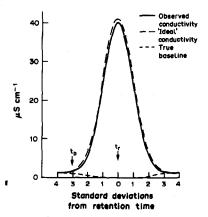
Fig. 6. Model ion-chromatographic peak for  $10 \,\mu$ mole of determinand with sodium tetraborate eluent.  $\lambda_{\text{borate}} = 37.4$ ,  $T_{\text{C}} = 0.018 M$ , otherwise notation as in Fig. 3).
