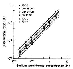
Fig. 3. Effect of sodium perchlorate concentration on the extraction of Co(II) by crown ethers (0.05M) in chloroform from aqueous perchlorate media at pH 5.2.
