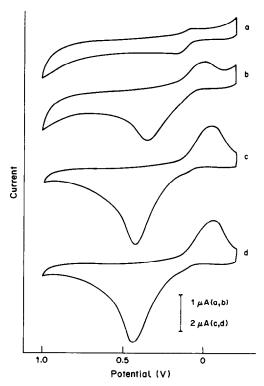
Fig. 4. Effect of film composition on the electrostatic uptake of dopamine. Cyclic voltamperograms for  $1 \times 10^{-4} M$  dopamine following 20-min accumulation. Nafion content (% v/v): (a) 16; (b) 25; (c) 37.5; (d) 100. The accumulation step was followed by transfer of the electrode to a blank (phosphate buffer) solution, for recording of the voltamperogram.
