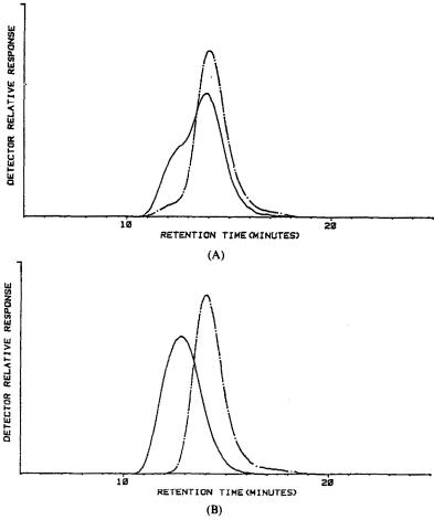
Fig. 25. Characterization of polystyrene-polycarbonate blend. (A) Normalized DRI (solid) and UV (dash) area-normalized gel-permeation chromatograms. (B) Calculated polystyrene (solid) and polycarbonate (dash) elution.
