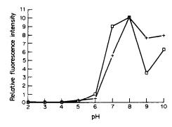
Fig. 5. Effect of pH on fluorescence yield (+ = methionine,  $\square$  = lysine).
