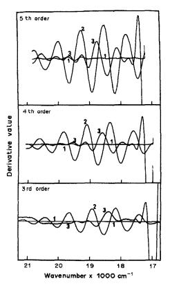
Fig. 2. Derivative absorption spectra of MnO<sub>4</sub> and Ni<sup>2+</sup> ions: 1, reagent blank; 2, 1  $\mu$ g/ml Mn; 3, 50 mg/ml Ni. Recording parameters: INT = 3, SPEED = 2,  $\Delta v = 60$  cm<sup>-1</sup>, EXP X = 2.
