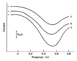
Fig. 5. Current-potential curves for the oxidation of  $4 \times 10^{-4} M$  hydrazine at CoPC/Nafion coated rotating-disk electrodes. Nafion content (% v/v): (a) 16; (b) 25; (c) 37.5. Supporting electrolyte, 0.05M phosphate buffer (pH 7.4); scan-rate 5 mV/sec.
