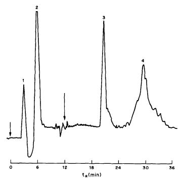
Fig. 4. Chromatogram of n-butyl acetate extract of phenol from aqueous solution. (1) n-butyl acetate, (2) phenol, (3) o-aminophenol, (4) m-aminophenol. Column Silasorb 600, 10 μm, 200 × 6 mm; 25°C; spectrophotometric detector (270 nm). Stepwise elution: n-hexane-butan-1-ol (97.5:2.5), after 12 min (85:15).
