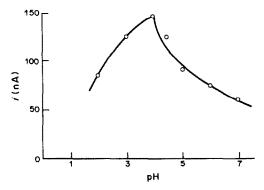
Fig. 8. Effect of pH on signal height for NO<sub>2</sub> determination. Nitrogen dioxide concentration 5.5 ppb; applied potential 1.0 V vs. Ag/AgCl; flow-rate 2.0 ml/min; injected sample size 136 μl; carrier supporting electrolyte 0.10M NaClO<sub>4</sub>.
