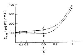
Fig. 8. Determination of platinum in the presence of titanium, palladium and ammonium ions in the air-acetylene flame. Test sample:  $100 \ \mu g \ Pt/ml$ , 3 mg Ti/ml, 3 mg Pd/ml and 3 mg NH<sub>4</sub> /ml. Curve A: without buffer interferent;  $c_{\rm App_{\infty}} = 100 \ \mu g/ml$ . Curve B: buffer interferent 5 mg La/ml;  $c_{\rm App_{\infty}} = 104 \ \mu g/ml$ .
