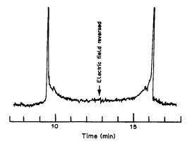
Fig. 3. Illustration of peak tailing due to a poor manual injection. Reversal of the electric field polarity at 12.8 min results in passage of the sample band through the UV detection region for a second time, producing of near "mirror image" of the peak.
