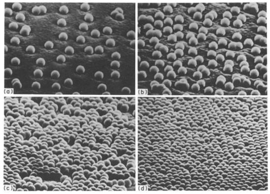
Fig. 1. Scanning electron micrographs (taken with an ISI DS 130 instrument) of silver-coated microsphere substrates (176-nm diameter spheres). Substrates prepared with: (a) 0.33%; (b) 1%; (c) 3.3%; and (d) 10% w/w suspensions.
