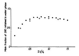
Fig. 3. Mole fraction of SXO remaining in water phase after t extraction stages with water from butanol and t stripping stages with butanol.  $V_{\rm W}/V_{\rm B}=0.1$  (extraction) and  $V_{\rm B}/V_{\rm W}=0.1$  (stripping) ( $\odot$ );  $V_{\rm W}/V_{\rm B}=0.25$  (extraction) and  $V_{\rm B}/V_{\rm W}=0.25$  (stripping) ( $\odot$ ). Both solvents were mutually saturated.
