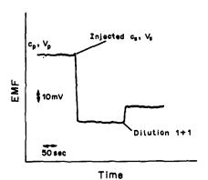
Fig. 3. Response time of cloxacillin electrode:  $c_p = 10^{-3} M$ ;  $c_s = 0.1 M$ ;  $v_p = 20 \text{ ml}$ ;  $v_s = 1 \text{ ml}$ ; dilution 1:1.
