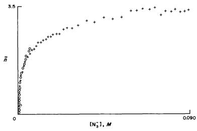
Fig. 1. Formation curve for the indium(III)-azide-system.  $C_{ln^{3+}}$ :  $\bigcirc$ ,  $3.69 \times 10^{-4}M$ ; +,  $9.83 \times 10^{-4}M$ .
