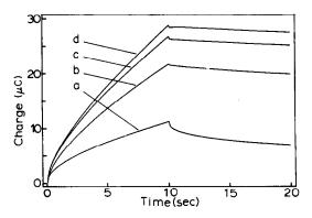
Fig. 3. Double potential-step chronocoulometry of metmyoglobin in the presence of various concentrations of oxygen. Metmyoglobin 81  $\mu$ M, potential steps from +0.520 V to -0.380 V (an overpotential of -426 mV). Oxygen concentration ( $\mu$ M): (a) 16, (b) 63, (c) 78 and (d) 94.
