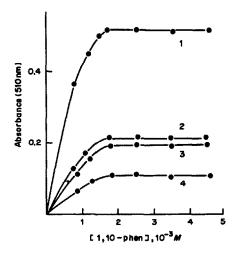
Fig. 4. Dependence of Fe(II)(phen)<sub>3</sub> yield on initial concentration of 1,10-phenanthroline. Conditions and curve numbers as for Figs. 2 and 3.
