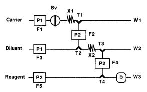
Fig. 1. Schematic of the cascade system manifold. P1 and P2 are peristaltic pumps,  $S_{\nu}$  is the injected sample volume, X1 and X2 are mixing coils,  $F_1$ - $F_4$  are flow-rates, D is the detector, and  $T_1$ - $T_4$  are the V-shaped connections.
