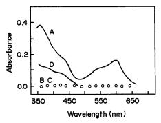
Fig. 1. Absorption spectra of DCE extract of the Fe(II)-TPTZ-pic complex and the binary combinations of the reactants, measured against DCE. (A) Fe-TPTZ-pic; (B) Fe(II)-TPTZ; (C) Fe(II)-pic; (D) TPTZ-pic.
