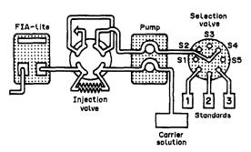
Fig. 6. Typical multipoint sampling application of the "FIA/lite" analyser.
