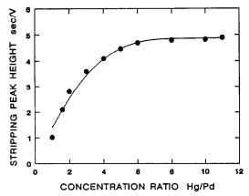
Fig. 2. Plot of stripping peak height vs.  $Hg^{2+}$  concentration during deposition. Conditions:  $1 \times 10^{-8} M$  Pd<sup>2+</sup>; others as for Fig. 1(b).
