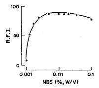
Fig. 1. Effect of NBS concentration on the fluorescence intensity: caffeine taken, 1.0  $\mu$ g.
