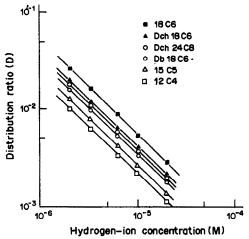
Fig. 1. Effect of the hydrogen-ion concentration on the extraction of Co(II) by crown ethers (0.05M) in chloroform from perchlorate aqueous media at constant ionic strength 0.1 (H<sup>+</sup>, NaClO<sub>4</sub>).
