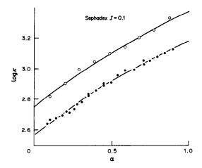
Fig. 1. Log  $\kappa$  plotted against  $\alpha$  for the system H<sup>+</sup>-Na<sup>+</sup> on Sephadex at 298.2 K. The ionic strength in the aqueous phase I = 0.100M (Na)ClO<sub>4</sub>.  $\bigcirc$  Sephadex C-25; ( Sephadex C-50. The curves were calculated from equation (5) with the parameters in Table 5.
