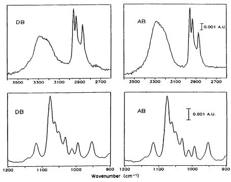
Fig. 4. Dual-beam spectra (DB) and absorbance spectra (AB) of n-butanol (5 monolayers) on nickel(100) at 150 K.
