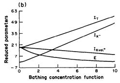
Fig. 2. Predicted behavior of limiting current vs. bathing electrolyte concentration: total current, anion current, cation current and electric field. (a) Symmetric bathing, flooded membrane; calculations with equations (6)–(8) with S=1, K=1,  $\bar{V}=10$ ,  $D_X/D_{Kval}=5$ . (b) Asymmetric bathing; calculations with equations (14) (18) and (19) with the same parameters as for (a).  $I_T=$  total current; field (-E) is  $(Fd/RT)\partial\phi/\partial x$ ; reduced currents are (-Id/FAD)
