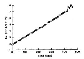
Fig. 3. Plot of the natural logarithm of the ratio of the instantaneous concentrations, vs. time. The intercept = 1.753 and the slope = 0.0127; the correlation coefficient for the regression is 0.9962. The second-order rate constant calculated from the slope is 0.457 1. mol<sup>-1</sup>. sec<sup>-1</sup>. Initial amount of sulphur 0.001728 mole and initial amount of tri-isopropyl phosphite 0.000297 mole. Volume 52 ml.
