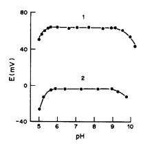
Fig. 2. Effect of pH on the potential of the oxacillin-CTOA electrode. Concentration of sodium oxacillin: 0.001M (1); 0.01M (2).
