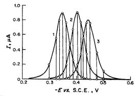
Fig. 3. Three selected experimental DP polarograms for the system Cu-morpholine (L).  $[Cu(II)] = 1.1 \times 10^{-5}M$ . 1, [L] = 0.056M; 2, [L] = 0.915M; 3, [L] = 1.521M. The points shown on the curves constitute part of the matrix **Z** (see text).
