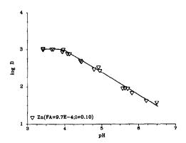
Fig. 2. The variation of the distribution coefficient (D) of Zn(II) in the presence of fulvic acid, as a function of pH.
