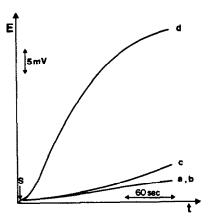
Fig. 4. Effect of pH on the reaction of FDNB  $(1.78 \times 10^{-3} M)$  with isoniazid  $(3.33 \times 10^{-3} M)$  at 25° (a) pH 6.0, (b) pH 7.0, (c) pH 8.0, (d) pH 9.0.
