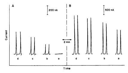
Fig. 8. Flow-injection peaks for ascorbic acid solutions containing increasing hydrazine concentrations, at the CoPC/Nafion (84/16% v/v) (A) and CoPC (B) coated electrodes: (a)  $1 \times 10^{-4}M$  ascorbic acid; (b-d) as for (a) but after successive additions of  $1 \times 10^{-4}M$  hydrazine. Applied potential, +0.70 V; other conditions as for Fig. 6.
