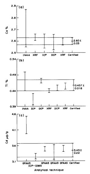
Fig. 3. The relationship of the certified value to results from individual analytical techniques. (a) Calcium—close agreement by all techniques. (b) Titanium—results by the technique using acid digestion (ICP) were eliminated in the determination of the certified value. (c) Cadmium—one result by the GFAAS technique was biased but results from other laboratories or techniques made certification possible.
