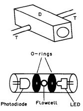
Fig. 6. LED-based, radial optical-path detector. The top portion shows the external appearance, a glass tube (flow-cell) TT passing through a \( \frac{1}{4} - 28 \) female coupler D. The internal placement of components is shown in the lower portion.
