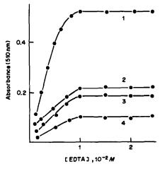
Fig. 2. Dependence of Fe(II) (phen)<sub>3</sub> yield on initial concentration of EDTA at pH 5.7 (acetate buffer), [MV<sup>2+</sup>] = 0.001M, [phen] = 0.004M, [Fe(III)] = 8 × 10<sup>-5</sup> M, diamino-acridine concentration 2 µm. Irradiation time 15 min: (1) proflavine and acriflavine, (2) Acridine Orange, (3) Acridine Yellow, (4) rivanol.
