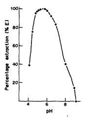
Fig. 1. Effect of pH on extraction of zinc.
