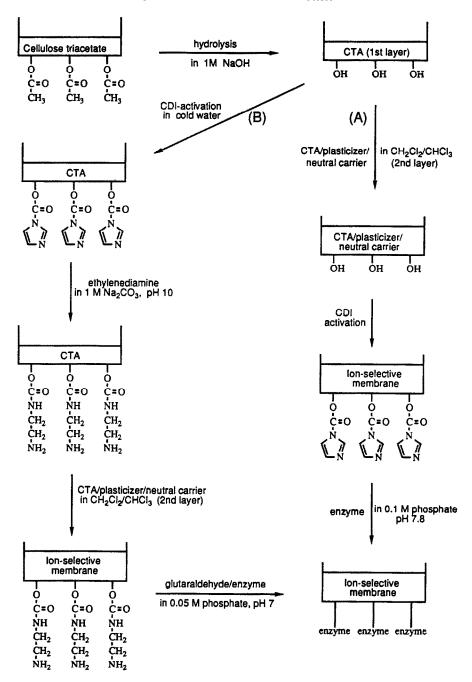
Fig. 1. General schemes used to prepare enzyme-immobilized asymmetric ion-selective cellulose triacetate membranes; (A) the direct CDI method for the hydroxylated membrane; (B) the glutaraldehyde method for aminated membrane.
