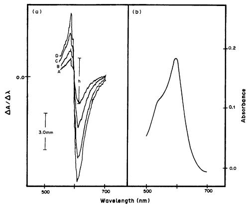
Fig. 5. (a) First-derivative spectra of DCE extract of the Fe-TPTZ-pic complex measured against a reagent blank; aqueous phase iron concentrations ( $\mu$ g/ml) (A) 0.012, (B) 0.024, (C) 0.036, (D) 0.048; all other conditions as in text; scan-speed 100 nm/min, 10-mm cells,  $\Delta\lambda = 2.0$  nm. (b) Absorption spectrum of DCE extract of the Fe-TPTZ-pic complex measured against a reagent blank. All other conditions as in text, but aqueous phase iron concentration 0.048  $\mu$ g/ml.
