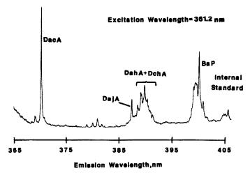
Fig. 2. Fluorescence spectrum of four-component dibenzacridine mixture in solid argon at the optimum excitation wavelength for dibenz[a, c] acridine. Benzo[a]pyrene was added as internal standard.
