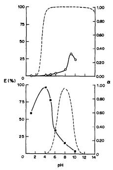
Fig. 2. Efficiencies for extraction of <sup>203</sup>Hg (○) and <sup>59</sup>Fe (■) with 0.25M HL in toluene, and fraction (α) of uncharged hydroxides (---), as a function of pH.
