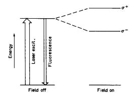
Fig. 1. Zeeman energy levels for an ac magnetic field parallel to the excitation beam.
