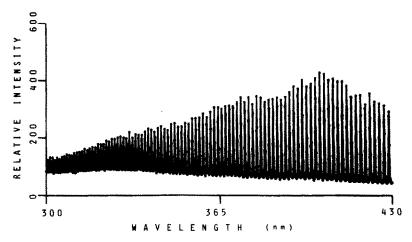
Fig. 4. Profile of the orders of an echelle spectrum for a continuum source.
