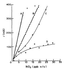
Fig. 7. Dependence of signal height on injected NO<sub>2</sub> concentration. (A) polymer-coated glassy-carbon electrode prepared with 10 cycles; (B) polymer-coated glassy-carbon electrode prepared with 120 cycles; (C) modified carbon paste electrode; (D) naked glassy-carbon electrode. Applied potential 1.0 V vs. Ag/AgCl. Flow-rate 2.0 ml/min. Injected sample size 250 μl. Carrier supporting electrolyte 0.10M KCl (pH 4.00).
