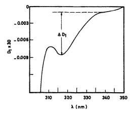
Fig. 3. First-derivative  $D_1$  curve of 1% aspirin solution containing salicylic acid. Correction of a constant interference. Horizontal line (---),  $\Delta D_1$  corrects for a constant interference.
