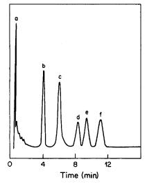
Fig. 1. Chromatogram of a mixture of iron(III), nickel(II), copper(II), mercury(II) and cobalt(II). The chromatogram is run on the radial compression cartridge column under the conditions described in the text. The metals are present at concentrations of about  $10\mu M$ .
