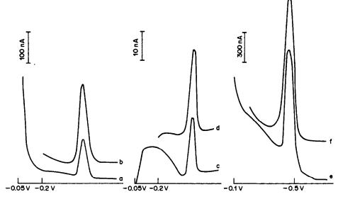
Fig. 2. Comparison of DP-AV (a, b) DC-AV (c, d) and LPS-AV (e, f) curves of  $5 \times 10^{-8} M$  Cu in 0.1 M ammonia buffer,  $5 \times 10^{-4} M$  nioxime, obtained in stirred solution at accumulation potentials of -0.2 V (curves b, d, f), -0.05 V (curves a, c) or -0.1 V (curve e):  $t_{acc} = 30$  sec.
