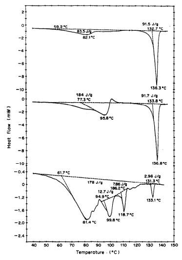
Fig. 23. Three DSC scans of different lots of the same pharmaceutical intermediate, taken on a commercial DSC.
