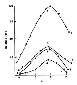
Fig. 1. Rate of photoreduction as a function of pH (relative to rate for proflavine at pH 6, assigned a value of 100): (1) proflavine and acriflavine, (2) Acridine Orange, (3) Acridine Yellow, (4) rivanol.
