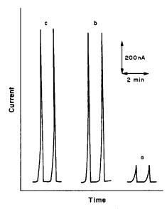
Fig. 6. Flow-injection peaks for  $5 \times 10^{-3} M$  hydrazine at the bare (a), CoPC(b) and CoPC/Nafion (75/25% v/v) (c) electrodes. Applied potential +0.45 V; supporting electrolyte, phosphate buffer (pH 7.4); flow-rate 1 ml/min.
