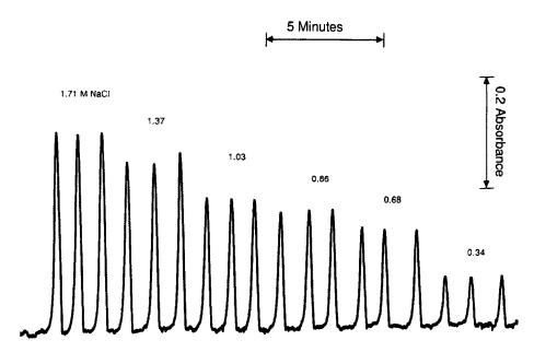
Fig. 7. Typical cascade system peaks. Given are triplicate injections with a calculated dilution factor of 470. Samples are 1.71, 1.37, 1.03, 0.86, 0.68, and 0.34M NaCl from left to right.
