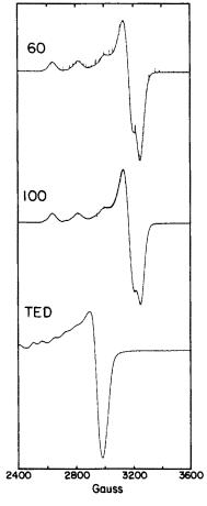
Fig. 4. EPR spectra for batch 860617089 of immobilized TED with Cu(II) equivalent to 60% and 100% of the experimental binding capacity. The spectrum designated TED is for the Cu(II) complex of the immobilized TED sample provided by the referee. Spectra recorded in MES buffer at a frequency of 9.15 GHz.
