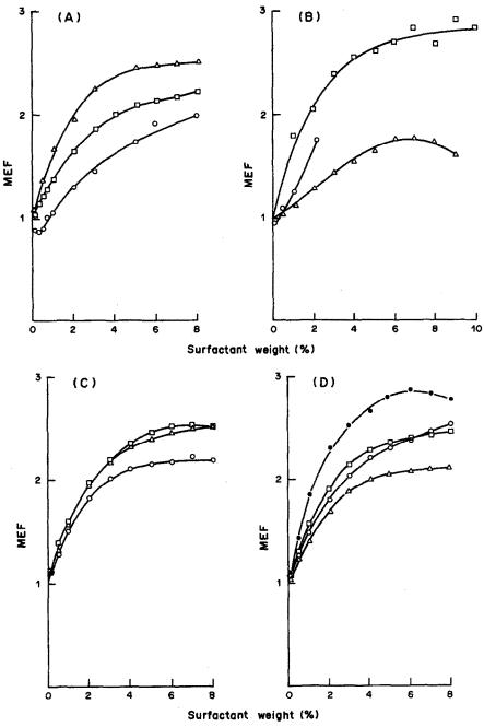
Fig. 2. Influence of the concentration of non-ionic surfactants on the MEF values of carbaryl at pH 12. A: Dehscoxid 728 □, Dehscoxid 729 △ and Dehscoxid 650 ○. B: Triton X-100 □, Triton X-114 ○ and Triton X-405 △, C: Nemol K-38 △, Nemol K-39 ○ and Nemol K-539 □. D: Nemol K-1030 ♠, Nemol K-1033 □, Nemol K-1035 △ and Nemol K-2030 ○. Concentration of carbaryl 5 ppm.
