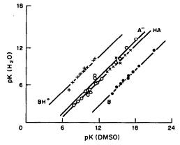
Fig. 6. Plot of pK-values in the studied DMSO/water mixture and in water for 56 differently charged acids and bases. The intercepts give the medium effects.
