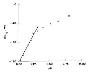
Fig. 2. Effect of pH on the half-wave potential of the TTA-wave. Aqueous-phase: 0.2M NaOAc. DCE phase: 0.01M THA · TPB, 0.4mM HTTA.
