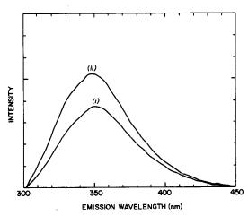
Fig. 4. Emission spectra of adsorbed lysozyme collected on initial contact (i) and after 90 sec incubation (ii). Conditions: excitation wavelength, 295 nm; band-width, 4 nm; scan-rate, 2.5 nm/sec; flow-rate, 0.3 ml/min; 1% methanol in 10 mM phosphoric acid, pH 2.3; temperature 4°C; 5 μg of lysozyme injected. Reproduced by permission from X-M. Lu, A. Figueroa and B. L. Karger, J. Am. Chem. Soc., 1988, 110, 1978, Copyright 1988, American Chemical Society.
