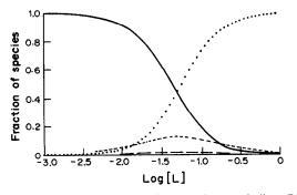
Fig. 5. Species distribution for the Cu-morpholine (L) system: ——, CuL; ..., CuL<sub>3</sub>; ——, CuL<sub>2</sub> ( $\beta_2 = 1.0 \times 10^{12}$ ); ---, CuL<sub>2</sub> ( $\beta_2 = 1.0 \times 10^{13}$ ). The CuL and CuL<sub>3</sub> values are those calculated with  $\beta_2 = 1.0 \times 10^{12}$  for CuL<sub>2</sub>.
