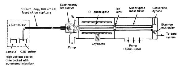
Fig. 1. Schematic illustration of the instrumentation for combined capillary electrophoresis-mass spectrometry.
