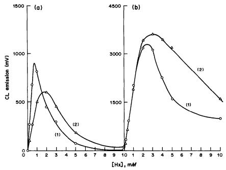
Fig. 3. Effect of hydroxylamine concentration at (a)  $[IO_4^-]_0 = 1.0 \times 10^{-3} M$  and (b)  $[IO_4^-]_0 = 1.0 \times 10^{-2} M$ . Conditions: pH 8.0;  $[Pg]_0$  5.0 × 10<sup>-4</sup> M (1), 1.0 × 10<sup>-3</sup> M (2).
