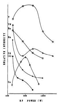
Fig. 3. The effect of rf power on the fluorescence signal for each element.
