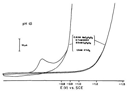
Fig. 2. Cyclic current-voltage curves for supporting electrolyte (0.85M sodium acetate, 67mM HEDP, 85mM ascorbic acid) and 1.0mM TcO<sub>4</sub> in supporting electrolyte; pH 4.5.
