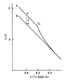
Fig. 1. Plot of ln k' vs. 1/T for an octyl phase. Mobile phase: water. Test solute: phenol. Evaluation cycle: (A) initial run, (B) rerun following thermal conditioning. Dashed line (C): Δ ln k', at 20°C (i.e., measurements of solute retention taken before (point a) and after (point b) surface reordering/resolvation).
