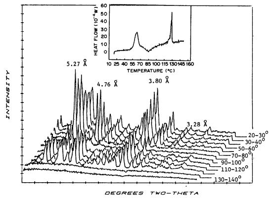
Fig. 24. DSC and XRD data for the pharmaceutical intermediate taken on the DSC/XRD instrument. In this DSC scan, endotherms point up. In Fig. 23, endotherms point down. The XRD plots are of intensity vs. 2 $\theta$  at the temperatures shown at the right-hand end of each plot.
