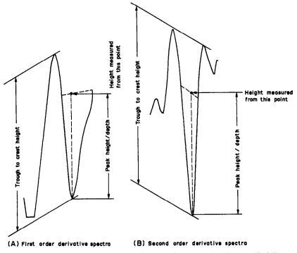
Fig. 3. Measurement of (A) first and (B) second order derivative spectra. In (A) the vertical distance from the crossover point to the trough is measured. In (B) a line is drawn between the crossover points and the vertical height from this line to the trough is measured.
