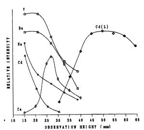
Fig. 2. The effect of observation height above the load coil on the fluorescence signal for each element.
