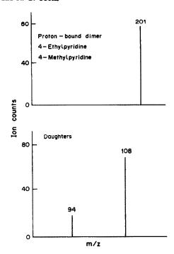
Fig. 4. Mass spectrum for the proton-bound dimer formed between 4-ethylpyridine and 4-methylpyridine, observed at m/z 201. It dissociates to compounds with m/z 108 and 94 after collisional activation.
