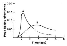
Fig. 15. Peaks of molybdenum as a function of atomization time in a graphite tube at 2800°. Curve A: without interferent. Curve B: in the presence of 0.5 mg V/ml (as vanadium chloride).
