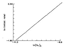
Fig. 2. Plot to determine the reaction order for NH<sub>3</sub>. Initial rates are determined from values of k'' returned by the nonlinear fitting routine. Slope = 1.023<sub>6</sub>. Standard error of the estimate = 0.019<sub>3</sub>. Variance of the slope =  $1.1 \times 10^{-4}$ .
