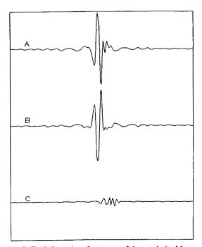
Fig. 2. Single-beam interferograms of the s-polarized beam (A), the p-polarized beam (B) and the resulting "optical null" interferogram (C).
