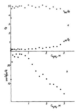
Fig. 1. Dependence of extraction coefficients on sulphuric acid concentration: (a) SXO  $(\bigcirc)$ , XO  $(\bigcirc)$ ; (b)  $_{\text{SXO}}D_{\text{E}}/_{\text{XO}}D_{\text{E}}$ .
