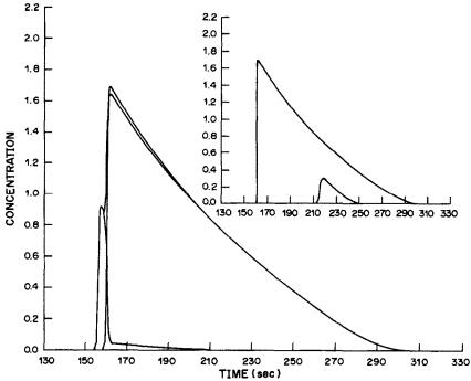
Fig. 8. Elution profile of a high concentration band (loading factor, 10%) of a binary mixture (relative retention at zero sample size, 1.09; same column capacity). Value of  $k'_0$  for the second compound, 6.25. Limit retention times of the two compounds, 290 and 270 sec, respectively.  $t_0 = 40$  sec. Relative concentration of the two compounds, 1/19. Insert: chromatograms obtained for the same amounts of each component injected singly.
