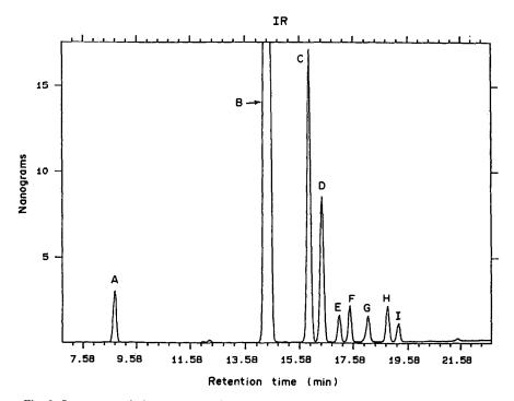
Fig. 8. Reconstructed chromatogram (infrared detector) of a mixture of substituted pyridines.
