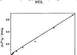
Fig. 8. Plot of  $[Cu^{2+}]_2/[CuL]_2$  vs.  $[Cu^{2+}]_2$  for the 4.0 mg/l. HA solution.
