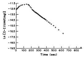
Fig. 11. Plot of  $ln[I-I_L]$  vs. time for the transient in Fig. 10. Slope = -10.8, y-intercept = -10.41, square correlation coefficient = 0.9977.
