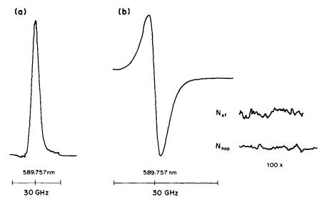
Fig. 2. Polarization signals for Na at 1.95  $\mu$ g/l. (a) Lorentzian signal for  $\theta = 0^{\circ}$ ; and (b) dispersion signal for  $\theta = 0.040^{\circ}$ . Noise in (b) is expanded  $100 \times$ .
