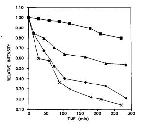
Fig. 1. Relative fluorescence intensity of Ag\*F (2.0 × 10<sup>-8</sup>M) in pH 7.4 TRIZMA buffer, in different cuvettes, as a function of time. (×) Polyethylene, (■) silica, (◆) polystyrene, (▲) poly(methyl methacrylate).
