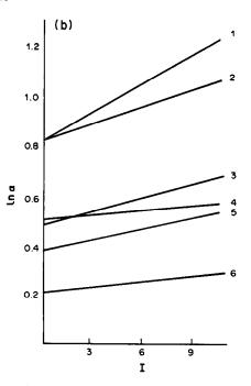
Fig. 5. (a) Plot of capacity factors against ionic strength of mobile phase: 1—uridine; 2—cytosine arabinoside; 3—cytidine; 4—6-azauridine; 5—6-azacytidine. (b) Plot of selectivity of separation of nucleosides against ionic strength of mobile phase: 1—uridine and 6-azauridine; 2—cytidine and 6-azacytidine; 3—uridine and cytidine; 4—6-azauridine and 6-azacytidine; 5—cytosine and cytidine arabinoside; 6—uridine and cytosine arabinoside.
