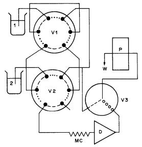
Fig. 3. A nested loop ACCAS system. V1, 2: PTFE rotary valves; V3: 3-way valve; other symbols as in Fig. 1.
