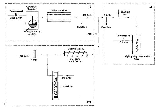
Fig. 2. Apparatus for the detection of chlorine and tetrachloroethene by means of an aerosol. I, Generation of the Rhodamine B aerosol. II, Generation of test-gas atmospheres of C<sub>2</sub>Cl<sub>4</sub> and Cl<sub>2</sub> by pemeation tubes.
