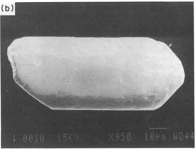
Fig. 2. Scanning electron microscope photographs of particles remaining after acid digestion of SRM 2704. (a) Rutile (TiO<sub>2</sub>). (b) Zircon (ZrSiO<sub>4</sub>).
