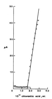
Fig. 1. Typical titration graph.
