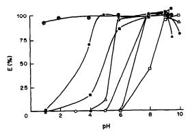
Fig. 1. Efficiencies for extraction of <sup>64</sup>Cu (⊕), <sup>60</sup>Co (●), <sup>65</sup>Ni (■), <sup>65</sup>Zn (△), Pb (○), <sup>56</sup>Mn (▲), and <sup>115</sup>Cd (□) with 0.25M HL in toluene, as a function of pH.
