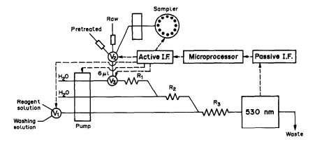
Fig. 8. Design of an automated analyser for determination of sulphate in concentrated phosphoric acid.<sup>35</sup>
