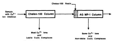
Fig. 1. Two-column ion-exchange measurement scheme.
