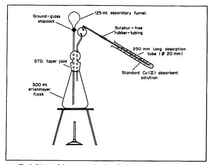
Fig. 1. Scheme of the apparatus for determination of sulphur by evolution.
