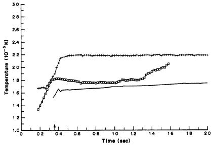
Fig. 3. The surface and vapour temperature profiles of SP-9 modified tube I during wall atomization at 2273 K Symbols as for Fig. 2
