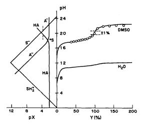
Fig. 7. Theoretical titration curves of sulphoguanidine in DMSO/water mixture and in water (full lines). The experimental data are shown with open circles.
