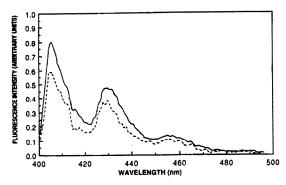
Fig. 5. Emission fluorescence spectra of benzo[a]pyrene: --- on filter paper; --- on paper treated with fumed silica.
