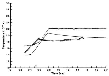
Fig. 2 The surface and vapour temperature profiles of the unmodified SP-9 tube with wall atomization at 2273 K, vapour ( $\square$ ), wall at the tube centre (+), wall at tube end (-) The arrow indicates the time corresponding to the signal maximum for lead
