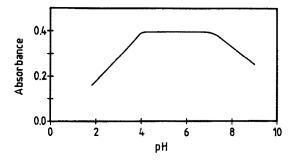
Fig. 4. Effect of pH on the formation and extraction of the complex. Absorbance measured at 600 nm against reagent blank, 10 μg of iron, 10 ml of 10<sup>-3</sup>M TPTZ, 4 ml of 0.01M picric acid, other conditions as for Fig. 2.
