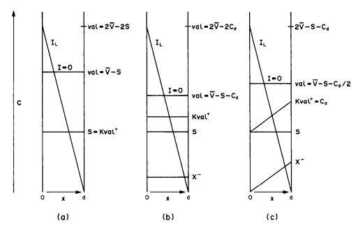
Fig. 1. (a) Schematic of concentration profiles of species in an ideal permselective carrier membrane at zero and at limiting current. (b) Schematic of concentration profiles of species in a symmetrically bathed, carrier membrane at failure of Donnan exclusion. (c) Schematic of concentration profiles of species in an asymmetrically bathed carrier membrane at zero and at limiting current, at failure of Donnan exclusion.
