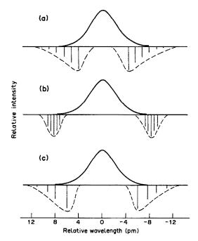
Fig. 2. Zeeman splitting patterns for Mn. The convolution of the laser emission profile and atomic spectra profile is shown along with the (inverted) calculated sigma component splitting pattern. (a) 279.5 nm  $(^6S_{5/2}^{-6}P_{7/2})$ , (b) 279.8 nm  $(^6S_{5/2}^{-6}P_{5/2})$ , (c) 280.1 nm  $(^6S_{1/2}^{-6}P_{3/2})$ .
