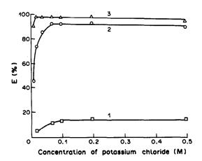
Fig. 3. Effect of aqueous phase concentration of potassium chloride on extraction of copper with tetra-alkylammonium ions. The initial concentration of tetra-alkylammonium ion in the aqueous phase is  $1 \times 10^{-3}M$ . 1, TPA+; 2, TBA+; 3, TAA+.
