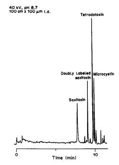
Fig. 5. Separation of fluorescamine-labeled toxins by CZE with fluorescence detection.
