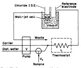
Fig 1 The flow-injection system used for the potentiometric determination of chloride
