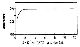
Fig. 3. Effect of TPTZ concentration on the formation and extraction of the complex. Absorbance measured at 600 nm against a reagent blank;  $10 \mu g$  of iron, 4 ml of 0.01M picric acid, other conditions as for Fig. 2.
