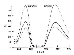
Fig. 1. Effect of pH on the excitation and emission RTP spectra of theobromine  $(10^{-3}M)$  on W-40 filter paper, in the presence of 1M KI: ——— neutral solution (sensitivity  $\times 0.8$ ); —— acidic (0.1M HCl) solution (sensitivity  $\times 1$ ); .... basic (1M NaOH) solution (sensitivity  $\times 5$ ).
