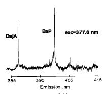
Fig. 6. Fluorescence spectrum of thirteen-component PAH mixture in solid argon at the optimum excitation wavelength for dibenz[a, j]acridine. Benzo[a]pyrene is used as internal standard.
