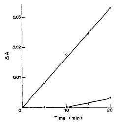
Fig. 1. Decomposition of Hg(II) dithizonate with time under 500-lux daylight irradiation. ●, CHCl<sub>3</sub>; ○, CCl<sub>4</sub>. Concentration of Hg(II) dithizonate = 1.4 μg/ml; initial absorbance = 0.098.
