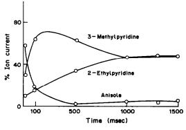
Fig. 3. The ion abundances for a 500:25:1 molar mixture of anisole, 3-methylpyridine and 2-ethylpyridine, as a function of time.
