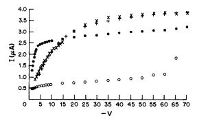
Fig. 4. Electrolyte concentration studies on the steady-state current-voltage properties of TDA membranes. Sweeps are in the direction of increasing voltages.  $\bigcirc$ , 0.1M HCl; \*, 0.01M HCl; +, 0.001M HCl;  $\times$ , 0.0001M HCl.
