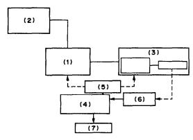
Fig. 9. Block diagram of an automated analyser for pharmaceutical dissolution tests (for details, see text).41
