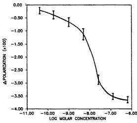
Fig. 7. Calibration curve for human insulin, with Ag\*F  $(5.2 \times 10^{-10} M)$  and Ab  $(4.0 \times 10^4 \text{ dilution})$  in pH 7.6 TRIZMA buffer with 0.025M NaSy.
