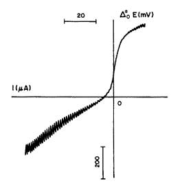
Fig. 1. Current-scan polarogram of HTTA. Aqueous phase: 0.2M NaOCa, pH 7.0 ± 0.1. DCE phase: 0.01M THA · TPB, 0.4mM HTTA.
