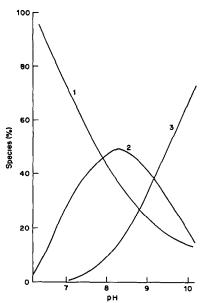
Fig. 3. Distribution of various species as a function of pH for the Zn-NTA-homocysteine system. (1) [Zn(NTA)]<sup>-</sup>, (2) [Zn(NTA)HL]<sup>2-</sup>, (3) [Zn(NTA)L]<sup>3-</sup>.
