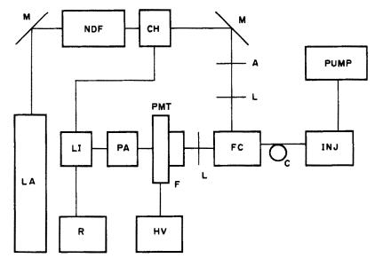
Fig. 1. Schematic of the laser-induced fluorescence detection system. LA, laser; M, mirror; NDF, neutral density filter; CH, chopper; LI, lock-in amplifier; PA, current-sensitive preamplifier; R, recorder; PMT, photomultiplier tube; HV, high-voltage supply; F, optical filter; L, lens; A, aperture; FC, capillary flow cell; C, capillary column.
