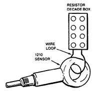
Fig. 4. Single-loop calibration circuit for measurement of cell constant (Foxboro MI 611-117, p. 24, Fig. 28).
