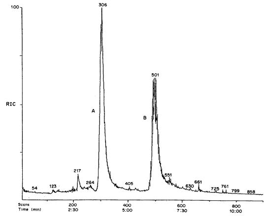
Fig. 1. LC/MS total ion chromatogram of a urine sample: column, 15 cm × 4.6 mm Spherisorb HPLC; eluent, H<sub>2</sub>O:CH<sub>3</sub>OH (60:40), 0.05*M* ammonium acetate, 0.01% acetic acid, 1 ml/min; post-column buffer, 0.5*M* ammonium formate in water, 0.3 ml/min.
