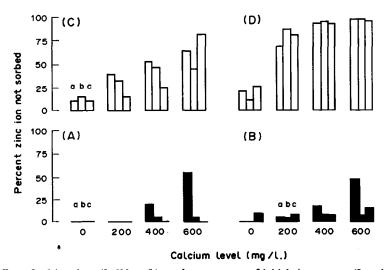
Fig. 1. Effect of calcium ions (0-600 mg/l.) on the percentage of initial zinc content (2 or 10 mg/l.) not taken up by ion-exchange resins of different types of forms. A, Strong acid, H<sup>+</sup>-form; B, strong acid, Na<sup>+</sup>-form; C, D, weak acid; WA2 and WA1, WA3, H<sup>+</sup>-form. Varying weights of exchanger (a, 200 mg; b, 500 mg, c, 1 g) added to 25 ml of Zn<sup>2+</sup>/Ca<sup>2+</sup> mixture.
