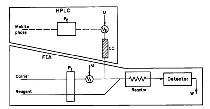
Fig. 12. Block diagram of HPLC-FIA coupling for rapid determination of analogous compounds. P, peristaltic pump; V, injection valve; M, sample; CC, chromatographic column; W, waste (for details, see text).
