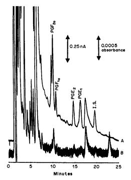
Fig. 4. Chromatogram of NPA derivatives of prostaglandins extracted from spiked urine sample. Chromatographic conditions: column, Supelcosil LC-8-DB, 15 cm × 4.6 mm; mobile phase, acetonitrile/50mM sodium acetate, pH 6 (50/50); flow, 1 ml/min. (A) HPLC-EC; detection, -0.90 V. (B) HPLC-UV; detection, 254 nm.
