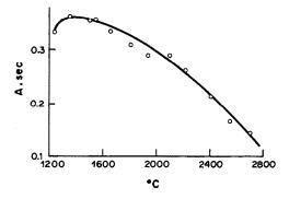
Fig. 6. The variation with temperature of the signal for Ag from 15  $\mu$ l of the NBS SRM 1643b Trace Metals in Water, 149 pg of Ag. The characteristic mass at the recommended atomization temperature of 1800° is 2.0 pg. (A.sec = absorbance.sec).
