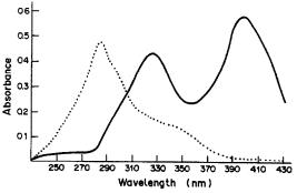
Fig. 1. Absorption spectra of the coloured product of picryl chloride with imipramine  $(4 \mu g/ml)$  — and reagent blank . . . . .
