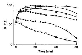
Fig. 2. Effects of reaction time and temperature of NBS on the fluorescence intensity: caffeine taken 1.0 µg; ○, 25°; ●, 30°; △, 35°; ■, 40°; △, 50°; □, 60°.
