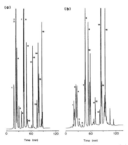
Fig. 6. (a) Chromatogram of standard amino-acid mixture (15 ng of each) (b) Chromatogram of hydrolysis products from 171 fmole of myoglobin. Peaks: (1) His; (2) Glu; (3) Gln; (4) Thr; (5) Asp; (6) Ser; (7) Tyr; (8) Gly; (9) Ala; (10) Arg; (11) Met; (12) Val; (13) Ile; (14) Leu; (15) Phe; (16) Lys.
