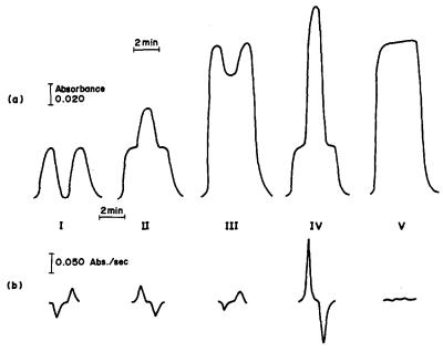
Fig. 3. (a) Normal and (b) derivative calibration recordings obtained from two different formaldehyde standards. Concentrations: I, standard 1  $\mu$ g/ml, sample 0  $\mu$ g/ml; II, standard 1  $\mu$ g/ml, sample 2  $\mu$ g/ml; IV, standard 1  $\mu$ g/ml, sample 4  $\mu$ g/ml; V, standard and sample both 3  $\mu$ g/ml.
