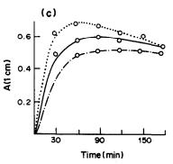
Fig. 5. Influence of heating time on the colour intensity developed from 1  $\mu$ mole of penicillin G sodium (a); 2  $\mu$ mole of ampicillin (b); 3  $\mu$ mole of cephalexin sodium (c) at various temperatures: 25° (——); 40° (...); 60° (----).
