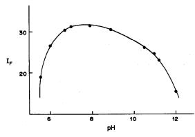
Fig. 2. Variation of the fluorescence intensity of the cadmium ion-association complex  $(C_{\rm Cd}=1.78\times 10^{-6}M)$  with pH;  $I_{\rm F}$  in arbitrary units.
