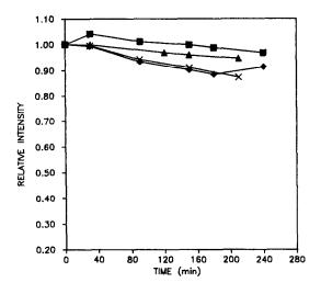
Fig. 2. Relative fluorescence intensity of Ag\*F (1.6 × 10<sup>-8</sup> M) in pH 7.6 TRIZMA buffer, in silica cuvettes, as a function of time. (♦) Buffer only, (▲) 10% ethanol, (×) 0.19mM RTX, (■) 0.025M NaSy.
