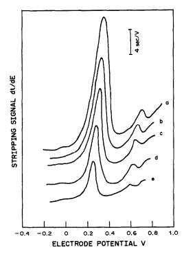
Fig. 4. Catalytic stripping signals of palladium. Deposition time 15 min. Other conditions as for Fig. 1(b). Pd<sup>2+</sup> concentration, (a) 0.9 pM, (b) 0.8 pM, (c) 7 pM, (d) 6 pM, (e) 5 pM.
