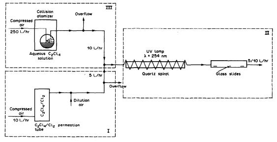
Fig. 1. Apparatus for the detection of chlorine and tetrachloroethene. I, Generation of test-gas atmospheres of  $C_2Cl_4$  and  $Cl_2$ . II, Combination of decomposition of  $C_2Cl_4$  and reaction of the chlorine produced, with immobilized Rhodamine B on glass slides. III, Transfer of  $C_2Cl_4$  into the gas phase by atomization of an aqueous solution.
