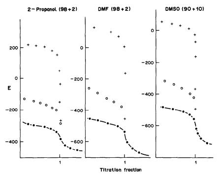
Fig. 2. Coulometric titration curves of  $HClO_4$  (×),  $MEAH^+$  (O), and the  $MEA + CO_2$  reaction product (•) in various solvents. Solid line—curve calculated for  $MEAH^+$  in presence of an excess of MEA.
