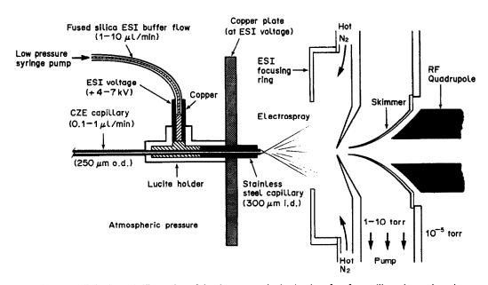
Fig. 2. Detailed schematic illustration of the electrospray ionization interface for capillary electrophoresis with mass spectrometry. A small-volume syringe pump is used to produce a liquid sheath electrode (ESI buffer).
