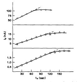
Fig. 3. Effect of preconcentration time on the stripping voltamperogram; ○, 10<sup>-6</sup>M; △ 10<sup>-7</sup>M; □, 10<sup>-8</sup>M nifedipine. Scan-rate 8.3 mV/sec. Britton-Robinson buffer (pH 4.4) 0.25M in NaClO<sub>4</sub>.
