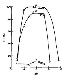
Fig. 1. Effect of pH on extraction of copper with tetraalkylammonium ions. The initial concentration of tetraalkylammonium ion in the aqueous phase is  $1 \times 10^{-3} M$ . 1, TPA<sup>+</sup>; 2, TBA<sup>+</sup>; 3, TAA<sup>+</sup>.
