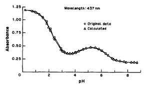
Fig. 2. Fit of observed and calculated absorbance vs. pH curves at 437 nm. Fluorescein,  $2.407 \times 10^{-5} M$ . Water only as solvent;  $\mu = 0.10$ . Calculation based on  $pK_{H_3F_1} = 2.19$ ,  $pK_{H_2F_1} = 4.24$ ,  $pK_{F_1} = 6.33$ .
