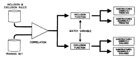
Fig. 2. Schematic of the rule-validation process. Inclusion and exclusion rules are correlated against each compound in the training set and the resulting predictions are categorized as correct or incorrect at various values of M.
