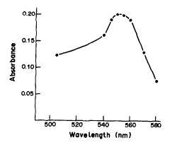
Fig. 3. Absorption spectrum of Zn-PAN complex in TPPO
