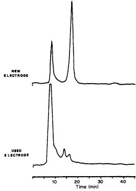
Fig. 10. The effect of "used" and "fresh" Hg on an electrochemically reduced <sup>99m</sup>Tc—HEDP mixture prepared at -1.200 V and pH 5.6.
