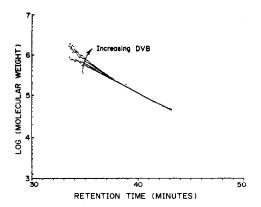
Fig. 27. Characterization of polymer crosslinking by gel permeation chromatography with light-scattering detection. Molecular weight determined vs. GPC retention for styrene-divinylbenzene copolymer (0, 78, 175, 325 ppm DVB).
