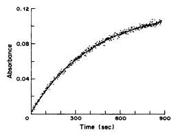
Fig. 8. Fit of a pseudo-first-order reaction model (solid line) to data collected for a reaction between phenol and chlorimine in the presence of SpF.
