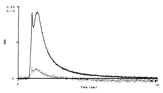
Fig. 4. The Cr absorbance profile demonstrating a split peak.
