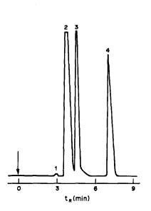
Fig. 7. Chromatogram of model mixture of benzene and monosubstituted phenols: (1) benzene, (2) σ-nitrophenol, (3) σ-chlorophenol, (4) σ-cresol. Column Silasorb 600, 10 μm, 200 × 6 mm; mobile phase 2.5% v/v butan-1-ol in n-hexane; 25°C; spectrophotometric detector (270 nm).
