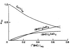
Fig. 5. The fraction of copper present in various complexes as a function of the total amine concentration. Lines were calculated with  $\log K'_{21} = 2.30$  and  $\log K'_{31} = 3.73$ .
