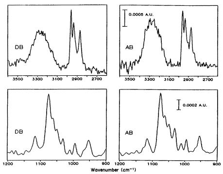
Fig. 5. Dual-beam spectra (DB) and absorbance spectra (AB) of n-butanol (1 monolayer) on nickel(100) at 150 K.
