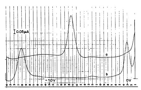
Fig. 3. Differential pulse polarograms obtained for (a) nifedipine solution at pH 6 in ethanolic phosphate buffer (30:70 v/v), (b) a nifedipine solution after irradiation.
