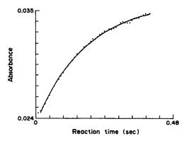
Fig. 4. Fit of a second-order reaction model (solid line) to absorbance data collected for the reaction of  $2.40 \times 10^{-4} M$  Cl<sub>T</sub> with  $1.20 \times 10^{-3} M$  N<sub>T</sub>. Solution absorbance data collected for the appearance of NH<sub>2</sub>Cl at 245 nm.  $k' = 2.467 \times 10^4$ . Average  $k_1 = 3.01 \times 10^6$ . Standard deviation =  $2.6 \times 10^3$ . Rate constant:  $k_1 = (3.0 \pm 0.3) \times 10^6$  1. mole<sup>-1</sup>, sec<sup>-1</sup>.
