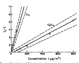
Fig. 4. Bleaching of Rhodamine B aerosol by gaseous Cl<sub>2</sub> and photolysed C<sub>2</sub>Cl<sub>4</sub> (relative humidity 35%). Regression lines and 95% confidence limits.
