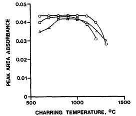
Fig. 2. Effect of ashing temperature on the integrated (peak/area) absorbance of 25  $\mu$ g/l. tin:  $\bigcirc$ , modifier A;  $\square$ , modifier B;  $\triangle$ , 5% modifier C.
