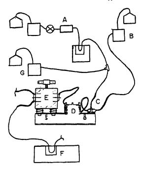
Fig. 13. Schematic representation of the RP-HPLC/FT-IR experiment with a membrane phase-separator and flow-cell interface.
