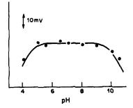
Fig. 4. Effect of pH on response of electrode to cloxacillin.
