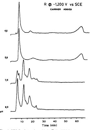
Fig. 6. HPLC of "carrier added"  $^{99m}$ Tc-HEDP mixtures prepared by coulometric reduction of TcO $_4^-$  at -1.200 V and various pH values. Conditions as for Fig. 5.
