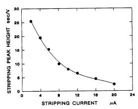
Fig. 3. Plot of stripping peak height vs. stripping current. Conditions as for Fig. 2.
