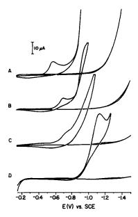
Fig. 3. Cyclic current-voltage curve for supporting electrolyte (same as for Fig. 2) and 1.0mM TcO<sub>4</sub><sup>-</sup> in supporting electrolyte at pH values of (A) 4.5, (B) 5.6, (C) 7.0 and (D) 9.0.
