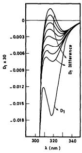
Fig. 4. First-derivative  $D_1$  curve of 1% solution of aspirin containing impurities other than salicylic acid,  $D_1$  difference curves obtained by compensation method with salicylic acid solutions of increasing concentrations in the reference cell. No balance point was obtainable.
