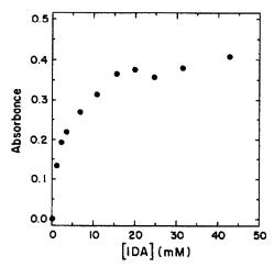
Fig. 3. Absorbance due to free copper, measured by AA, as a function of the amount of IDA added to a slurry of immobilized TED.
