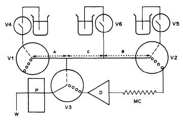
Fig. 2. Injecting multiple contiguous segments with a split loop. V4-V6 on/off valves; other symbols as in Fig. 1.
