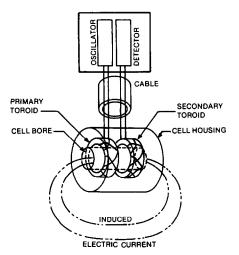
Fig. 1. Principle of the electrodeless conductivity cell and instrument.
