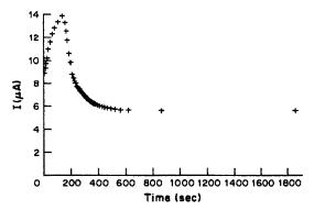
Fig. 10. Current-time decay of a 10.1mM ETH 1001 membrane in 0.001M CaCl<sub>2</sub>. Bias is -8.73 V.
