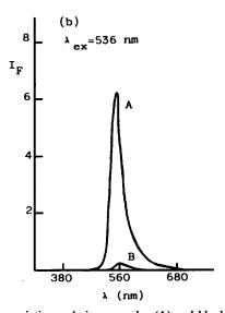
Fig. 1. Excitation (a) and emission (b) spectra of ion-association cadmium complex (A) and blank (B);  $I_F$  in arbitrary units.
