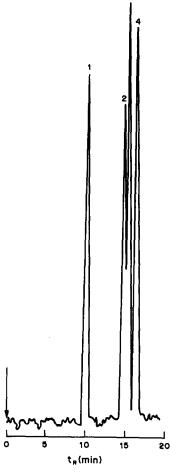
Fig. 3. Chromatograms of model mixture of cresols and phenol: (1) o-cresol, (2) m-cresol, (3) p-cresol, (4) phenol. Column Silasorb 600,  $6 \mu m$ ,  $120 \times 2 mm$ ; mobile phase 40% v/v chloroform in n-hexane; 25°C; spectrophotometric detector (270 nm).
