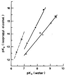
Fig. 1. Resolution of acid strength in isopropyl alcohol vs. water for several phenol derivatives. △ 4-Nitrophenol; × 3-nitrophenol; ○ 3,5-dichlorophenol; ○ 3-bromophenol; □ 4-chlorophenol; ★ 4-bromophenol; ▲ 2-nitrophenol; ● 2,4-dichlorophenol; ★ 2,4,6-trichlorophenol; ☆ 2,6-dichlorophenol.
