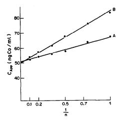
Fig. 13. Determination of cobalt in the presence of magnesium in a graphite tube at 2400°. Test sample: 50 ng Co/ml and 2 mg Mg/ml (as magnesium chloride). Curve A: sample in 1M hydrochloric acid;  $c_{App_{\infty}} = 51$  ng/ml. Curve B: sample in 0.5M nitric acid;  $c_{App_{\infty}} = 50$  ng/ml.
