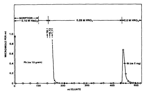
Fig. 1. Elution curve for Pb(II)-Bi(III): 5.0 ml of Chelex 100, H<sup>+</sup>-form, 100-200 mesh; column length 53 mm, diameter 11.0 mm; flow-rate 3.8 ± 0.3 ml/min.
