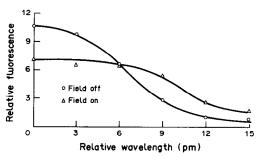
Fig. 3. Excitation wavelength scans for silver,  $(\bigcirc)$  without application of a magnetic field,  $(\triangle)$  with an applied field of 12 kG.
