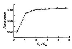
Fig. 4. Molar ratio plot for the Pd(II)-NMP system measured at 415 nm.  $C_M = 9.37 \times 10^{-6} M$ ; pH = 3.5.
