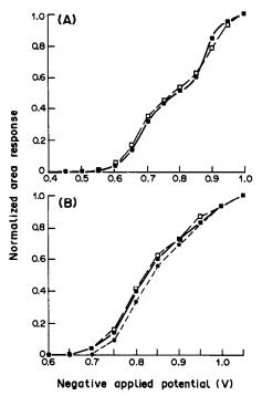
Fig. 2. Hydrodynamic voltamperograms of (A) DNPH and (B) NPA derivatives: (■) PGE<sub>2</sub>, (□) PGE<sub>1</sub>, (●) hexanoic acid.
