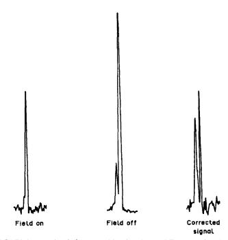
Fig. 6. ZETA-LEAFS furnace signals for 5-ng/ml Mn in a 1-mg/ml ZnCl<sub>2</sub> matrix. The "field on" signal is mostly due to scatter. The "field off" signal is analyte atomic fluorescence + scatter. The subtraction of the "field on" signal from the "field off" signal results in the corrected signal.
