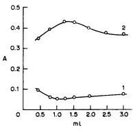
Fig. 3. Variation of the reaction rate with amount of hydrogen peroxide. (1) Uncatalysed reaction; (2) catalysed reaction; 1.0  $\mu$ g of Fe(III) per 25 ml.
