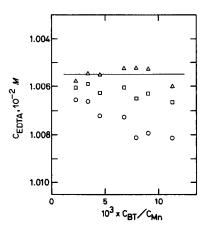
Fig. 2. Dependence (on indicator concentration) of the EDTA concentrations obtained by the three methods, for the manganese(II)-BT system.  $C_{\rm Mn}=1.625\times 10^{-3}M$  at the equivalence-points.  $\bigcirc$ , calculated from the inflexion point;  $\triangle$ , calculated from the equivalence-point by equation (8);  $\square$ , calculated from the equivalence-point by equation (6e).
