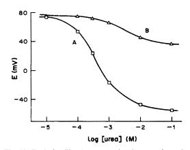
Fig. 10. Typical calibration curves for the urea electrodes prepared by using aminated H<sup>+</sup>-selective cellulose triacetate membranes. Urease was attached by one-step glutaraldehyde method (curve A) or two-step glutaraldehyde method (curve B). Potential measurements were made in 0.001M Tris-HCl/0.1M NaCl, pH 7.0.
