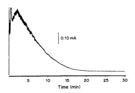
Fig. 4. Current-time response for coulometric reduction of  $TcO_4^-$  at -0.900~V~vs. SSCE. Same conditions as for Fig. 2.
