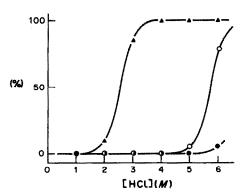
Fig. 3. Degree of extraction percentage of (▲) tellurium(IV), (○) selenium(IV) and (●) arsenic(V) into MIBK as a function of acidity of the aqueous phase.
