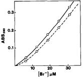
Fig. 3. Depression of standard curve caused by dissolved organic carbon (OC).  $\bigcirc -\bigcirc$ , [OC] = 0 mg/l.;  $\bigcirc ----\bigcirc$ , [OC] = 1.5 mg/l.
