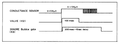
Fig. 8. Event diagram for pulsed reagent-introduction.
