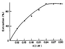
Fig. 2. Effect of potassium iodide concentration.
