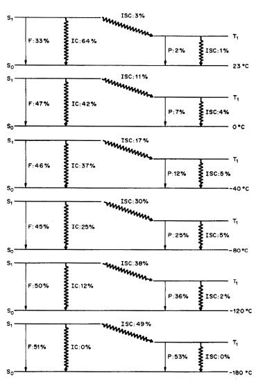
Fig. 1. Energy diagrams for 4-phenylphenol adsorbed on filter paper at different temperatures. S<sub>0</sub>—ground state, S<sub>1</sub>—singlet state, T<sub>1</sub>—triplet state, F—fluorescence, IC—internal conversion, ISC—intersystem crossing, P—phosphorescence.
