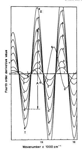
Fig. 4. Fourth-derivative spectra of  $MnO_4^-$  ion used for the calibration graph in the peak-to-trough technique: 1, reagent blank; 2-8, 0.125, 0.25, 0.50, 0.75, 1.0, 1.25 and 1.50  $\mu$ g/ml Mn, respectively; 9, 50 mg/ml Ni.
