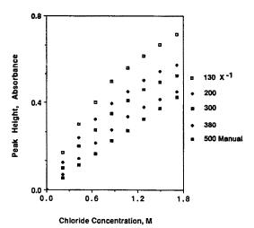
Fig. 6. Peak height vs. concentration for calculated X<sup>-1</sup> [by equation (4)] values of 130, 200, 300, and 380, and for 500-fold manually diluted samples injected into F<sub>4</sub>.
