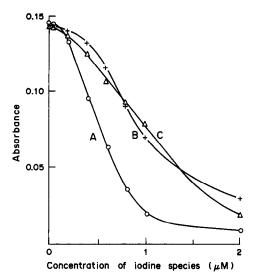
Fig. 2. Calibration curves for  $I^-(A)$ ,  $IO_3^-(B)$  and  $I_2(C)$ . For  $I_2$  the molar concentrations were half the values indicated. The concentrations of Hg(II) and Sn(II) were  $0.04\mu M$  and 6mM, respectively.
