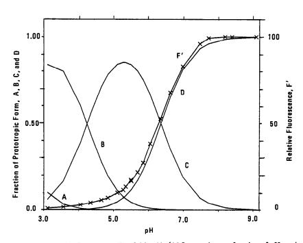
Fig. 1. Normalized relative fluorescence  $F_m'$  of  $6.0 \times 10^{-6} M$  fluorescein as a function of pH; excitation at 489 nm, emission at 516 nm, ionic strength  $\mu = 0.10$ . A, B, C and D are the fractions of fluorescein present as  $H_3Fl^+$ ,  $H_2Fl$ ,  $HFl^-$  and  $Fl^{2-}$  respectively as calculated from  $pK_{H_3Fl} = 2.19$ ,  $pK_{H_2Fl} = 4.24$ ,  $pK_{H_2Fl} = 6.36$ .
