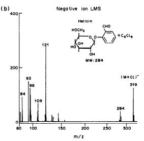
Fig. 6. Negative-ion LMS of (a) phenyl- $\beta$ -glucopyranoside, (b) helicin, mixed with hexachlorobenzene.
