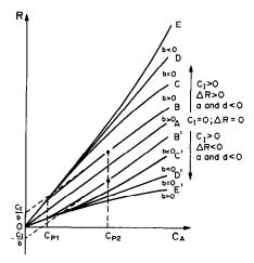
Fig. 1. Various types of interferent effects on the calibration curve.
