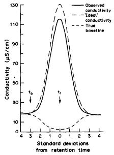
Fig. 3. Model ion-chromatographic peak for  $10 \,\mu$ mole of determinand with carbonate eluent, showing observed conductivity, "ideal" conductivity and true baseline:  $t_r$  = retention time,  $t_b$  = breakthrough time,  $\lambda_H$  = 350,  $\lambda_X$  = 75,  $\lambda_{HCO_3}$  = 44.5, V = 0.1 ml, F = 1 ml/min,  $T_C$  = 0.00505M.
