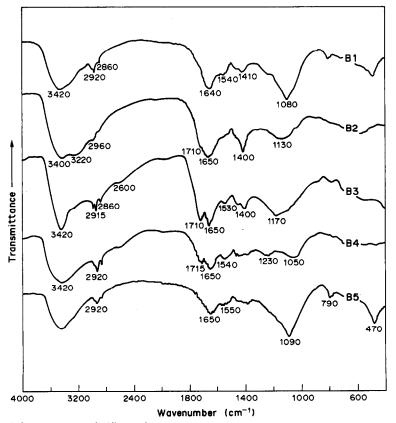
Fig. 3. Infrared spectra of different fractions of brewery sludge. Fraction numbers as in Fig. 1.
