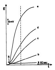
Fig. 1. Typical E-t curves of the FDNB-azide reaction for the calculation of the kinetic parameters and calibration graphs at 25° and pH 9.0. [FDNB] =  $1.78 \times 10^{-3} M$ ; [Azide] (a) blank, (b)  $6.67 \times 10^{-4} M$ , (c)  $3.33 \times 10^{-3} M$ , (d)  $6.67 \times 10^{-3} M$ , (e)  $3.33 \times 10^{-2} M$ . Dashed line shows the  $\Delta E$  measurement in the fixed-time method.
