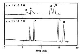
Fig. 8. Illustration of the effect of buffer ionic strength on CZE separation quality.
