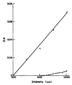
Fig. 2. Decomposition of Hg(II) dithizonate under daylight irradiation of varying intensities for 15 min: ♠, CHCl<sub>3</sub>; ○, CCl<sub>4</sub>. Concentration of Hg(II) dithizonate = 1.4 μg/ml; initial absorbance = 0.098.
