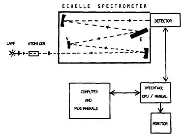
Fig. 1. Block diagram of the echelle-spectrometer/image-dissector system as used in this work. E, echelle grating; V, order-sorting grating.
