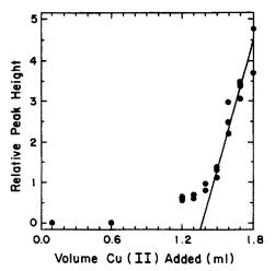
Fig. 2. Relative peak current measured by ASV as a function of the volume of Cu(II) solution added to a slurry of immobilized TED.
