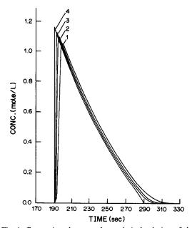
Fig. 1. Comparison between the analytical solution of the ideal model (infinite efficiency column) and the numerical solutions of the semi-ideal model, for different values of the column efficiency. Loading factor, 0.05. 1, Ideal model band profile; 2, 4000 plate column; 3, 2000 plate column; 4, 1000 plate column.
