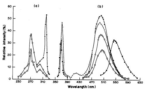
Fig. 1. Fluorescence spectra of the oxidation products of thioxanthenes: (a) excitation spectra; (b) emission spectra. □—□ Chlorprothixene (0.3 μg/ml). ●—● Thiothixene (0.55 μg/ml). ○—○ Clopenthixol.2HCl (0.4 μg/ml). ■—■ Methixene.HCl (0.32 μg/ml). ×—× Flupentixol.2HCl (0.27 μg/ml).
