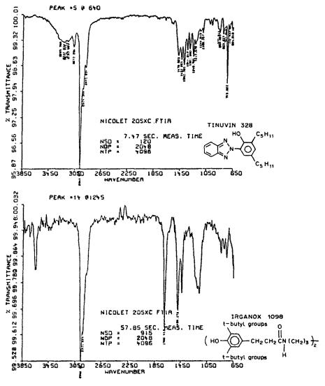
Fig. 11. Infrared spectra of two components shown in Fig. 3, obtained by GC/FT-IR analysis with a 1-m capillary column and high lightpipe interface temperatures.
