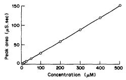
Fig. 5. Calibration for a model system ( $\lambda_{\rm H}=350,\ \lambda_{\rm X}=75,\ \lambda_{\rm HCO_3}=44.5,\ V=0.025\ {\rm ml},\ F=1.22\ {\rm ml/min}).$
