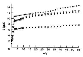
Fig. 6. Steady-state current-voltage curves for ETH 1001 membranes bathed in different concentrations of CaCl<sub>2</sub>: +, 16.0mM ETH 1001 membrane in 0.1M CaCl<sub>2</sub>; \*, 16.0mM ETH 1001 membrane in 0.01M CaCl<sub>2</sub>; O, 16.0mM ETH 1001 membrane in 0.001M CaCl<sub>2</sub>; ×, 10.1mM ETH 1001 membrane in 0.0001M CaCl<sub>2</sub>.
