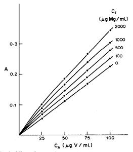
Fig. 2. Effect of magnesium on the calibration curve for vanadium in the nitrous oxide-acetylene flame.
