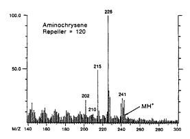
Fig. 6. TSP mass spectrum obtained from aminochrysene at two repeller voltages. Upper spectrum exhibits little fragmentation at 60 V whereas extensive fragmentation is produced at 120 V lower spectrum).
