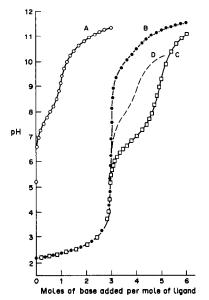
Fig. 1. Potentiometric titration curves for the Zn<sup>2+</sup>-NTA-PSH system, A—PSH; B—Zn<sup>2+</sup>:NTA; C—Zn<sup>2+</sup>:NTA:PSH and D—calculated curve.
