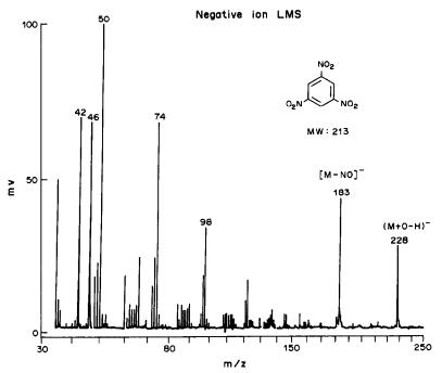
Fig. 1. Negative-ion laser mass spectrometry of 1,3,5-trinitrobenzene.
