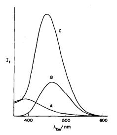
Fig. 1. Emission spectra (excitation wavelength 336 nm) of an alkaline aqueous solution of A, Nemol K-1030; B, carbaryl; C, carbaryl in the presence of Nemol K-1030.
