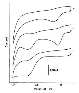
Fig. 1. Cyclic voltamperograms for a solution containing  $2 \times 10^{-4} M$  ascorbic acid and  $1 \times 10^{-3} M$  hydrogen peroxide, recorded at bare (a), CoPC-coated (b) and CoPC/Nafion (84/16% v/v) coated (c) glassy-carbon electrodes. Supporting electrolyte, 0.05M phosphate buffer (pH 7.4); scan-rate 100 mV/sec.
