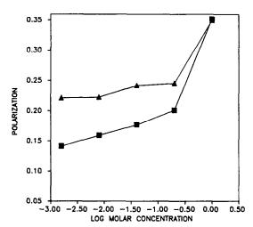
Fig. 4. Polarization of Ag\*F  $(7.8 \times 10^{-10} M)$  in pH 7.6 TRIZMA buffer as a function of NaSy concentration. Symbols as for Fig. 3.
