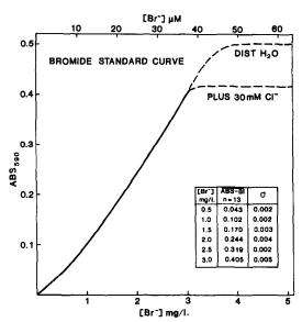
Fig. 2. Standard curve obtained with a CT concentration of  $38.6 \mu M$ .
