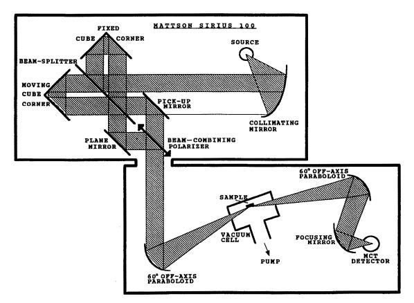
Fig. 1. Optical diagram of a differential polarization dual-beam FT-IR spectrometer.
