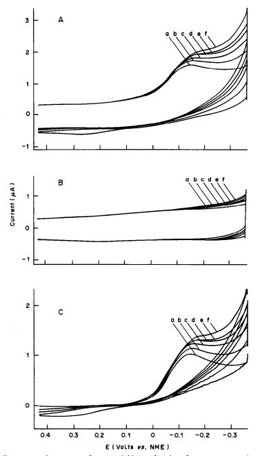
Fig. 1. Cyclic current-voltage curves of metmyoglobin as a function of oxygen concentration. Scan-rate = 50 mV/sec, electrode area =  $0.30 \text{ cm}^2$ . (A) Solution of  $61\mu M$  metmyoglobin in tris/cacodylic acid buffer, pH 7.0; (B) buffer alone; (C) background-subtracted cyclic current-voltage curves obtained by taking the difference between results shown in (A) and (B). In each case the oxygen concentrations  $(\mu M)$  are:
