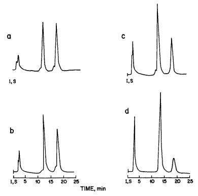
Fig. 2. Chromatographic behavior of papain as a function of the l-propanol concentration in mobile phase A with constant surface contact time. a = 0% propanol; b = 1.8% l-propanol; c = 3.6% l-propanol; d = 5.4% l-propanol. Other conditions: see Fig. 1. Reproduced from K. P. Benedek, S. Dong and B. L. Karger, J. Chromatog., 1986, 317, 227, by permission. Copyright 1986, Elsevier Science Publishers.
