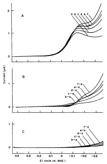
Fig. 2. Linear-sweep current-voltage curves taken from Fig. 1. (A) From Fig. 1(C); (B) background-subtracted negative linear-sweep current-voltage curves obtained by subtraction of trace (a) in (A) from each other trace to show only oxygen reduction; (C) background-subtracted negative linear-sweep current-voltage curves obtained by subtraction of trace (a) in Fig. 1(B) from each other trace.
