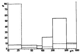
Fig. 1. Distribution of particle sizes for Zn<sub>2</sub>Fe(CN)<sub>6</sub> (continuous lines) and Na<sub>2</sub>Zn<sub>3</sub>[Fe(CN)<sub>6</sub>]<sub>2</sub> (dashed lines).
