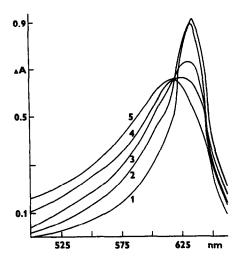
Fig. 3. Absorption spectra as a function of CAB concentration, at pH 5.6.  $c_{\rm M}=7\times10^{-6}M$ ,  $c_{\rm L}=7\times10^{-6}-7\times10^{-5}M$ ,  $c_{\rm T}=1\times10^{-3}M$ , 5% v/v ethanol, I=0.05  $c_{\rm L}/c_{\rm M}$ : 1, 1.0; 2, 2.0; 3, 3.5; 4, 5.0; 5, 10.0.
