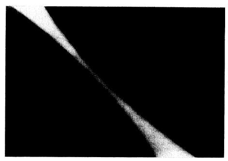
Fig. 5. Transmission electron micrograph of BN-×4 beads, 36,000 × magnification.
