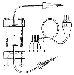
Fig 1 Flow-through tubular electrode design. (1) Perspex tube, (2) silver-loaded conductive epoxy resin, (3) flow channel (0 7 mm i.d.); (4) sensor membrane (0 5 mm thickness), (5) shielded electrical cable; (6) Perspex support pieces for connection to the manifold.
