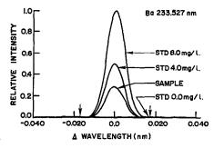
Fig. 1. An ICP-AES spectral scan of Ba at 233.527 nm.
