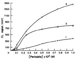
Fig. 4. Periodate calibration curves at constant [Hx]. Conditions: [Hx]<sub>0</sub>  $1.0 \times 10^{-3} M$ ; pH 8.0; [Pg]<sub>0</sub>  $2.5 \times 10^{-3} M$  (1),  $1.0 \times 10^{-3} M$  (2),  $5.0 \times 10^{-4} M$  (3).
