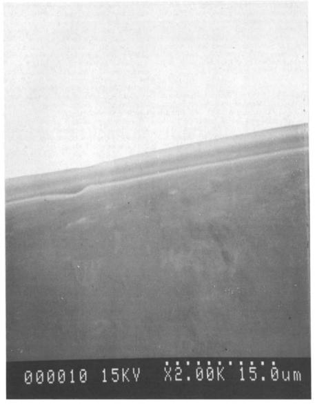
Fig. 2. Scanning electron micrograph showing the cross-section of a typical asymmetric ion-selective cellulose triacetate membrane.
