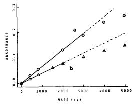
Fig. 5. Comparison of calibration curves for chromium (425.4 nm) by (a) the instrument described in this work, (b) the instrument previously described.
