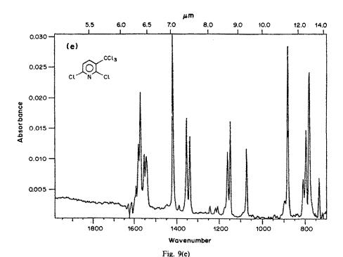
Fig. 9. Infrared spectra (2000–700 cm<sup>-1</sup>) of (a) peak E, 2,6-dichloro-4-trichloromethylpyridine, (b) peak F, 2,3-dichloro-5-trichloromethylpyridine, (c) peak G, 2,4-dichloro-5-trichloromethylpyridine, (d) peak H, 3,6-dichloro-2-trichloromethylpyridine, (e) peak I, 2,6-dichloro-3-trichloromethylpyridine.
