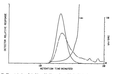
Fig. 26. Characterization of vinylidene chloride copolymer dehydrochlorination. Area normalized UV (dash) and DRI (solid) gel-permeation chromatograms, and dependence of UV/DRI response ratio on GPC retention index.
