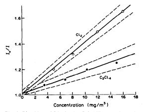
Fig. 3. Bleaching of Rhodamine B in silicone polymer by gaseous  $Cl_2$  and photolysed  $C_2Cl_4$ . Dotted lines: confidence limits (p = 0.95) of the regression line.
