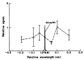
Fig. 5. Scatter signal as a function of excitation wavelength for a  $10-\mu l$  aliquot of a 1 mg/ml solution of ZnCl<sub>2</sub>. The error bars represent 1 standard deviation of the measurement. An ETA-LEAFS atomic spectral profile for 50 pg of Mn is shown for comparison.
