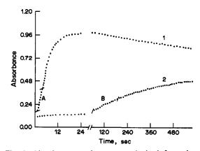
Fig. 1. Absorbance vs. time curves obtained from the stopped-flow determination of 25  $\mu$ g/ml 1-naphthol (1) and 2-naphthol (2). Zones A and B allow the reaction rates of 1-naphthol and 2-naphthol, respectively, to be determined. Experimental conditions as described in procedure.
