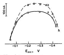
Fig. 6. Effect of the preconcentration potential on the DP-AV peak current for copper. Supporting electrolyte: 0.1M ammonia buffer,  $5 \times 10^{-4}M$  nioxime. Preconcentration time 60 sec. (a) Blank solution spiked with  $5 \times 10^{-8}M$  Cu. (b) Spring water spiked with  $6.5 \times 10^{-8}M$  Cu.
