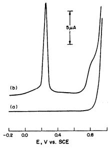
Fig. 2. Stripping voltamperogram of silver, obtained with a CMCPE. Reduction for 1 min at -0.2 V in 0.1M acetate buffer solution after accumulation for 1 min from 0.1M sodium perchlorate containing (a) 0, (b)  $10\mu M$  Ag(I). Scan-rate 50 mV/sec.
