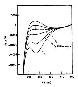
Fig. 2. First-derivative  $D_1$  curve due to salicylic acid present in 1% aspirin solution.  $D_1$ , difference curves obtained by the compensation method, with salicylic acid solutions of increasing concentrations in the reference cell, and first-derivative curve for pure aspirin (Z) obtained at the balance point after compensating for the total salicylic acid content in the sample solution.
