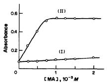
Fig. 2. Effect of mandelic acid concentration: (I), reagent blank; (II), net absorbance (Ge =  $4.1 \times 10^{-6}M$ ); Malachite Green,  $5.0 \times 10^{-4}M$ ; pH, 3.0.
