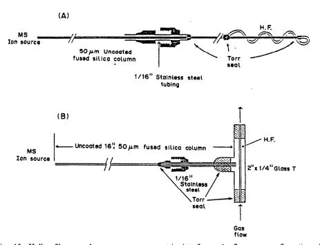
Fig. 15. Hollow-fiber membrane mass spectrometric interfaces: A, flow-over configuration; B, flow-through configuration (0.020 in. i.d., 0.037 in. o.d. Silastic medical grade tubing from Dow Corning).
