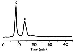
Fig. 12. HPLC of "no carrier added" <sup>99m</sup>Tc-HEDP mixture prepared by coulometric reduction at -1.200 V and pH 7.0. Conditions as for Fig. 5.
