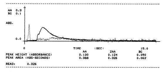
Fig. 5. A Cr absorbance profile on the Zeeman/3030 when improper drying conditions produced a large, early-running background peak.
