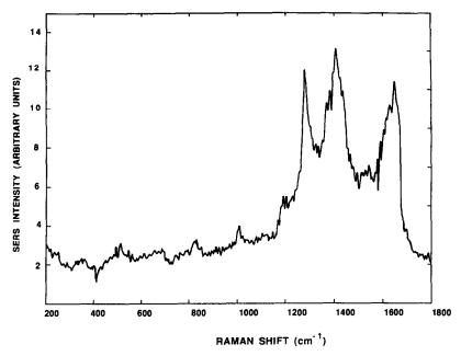
Fig. 4. In situ SERS spectrum of henzo[a]pyrene r-7, t-8, 9, 10-tetrahydrotetrol in solution.
