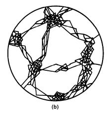
Fig. 1. Schematic representation of cross-linked (a) microporous resins (gels), average pore size 6-30 Å and (b) macroporous resins, average pore size 50-350 Å.
