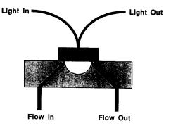
Fig. 2. Illustration of the reflected-transmittance flow cell.
