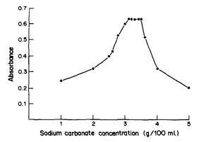
Fig. 3. Effect of concentration of sodium carbonate on the intensity of coloured reaction product of the ophylline (10  $\mu$ g/ml) with diazotized p-nitroaniline.
