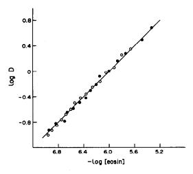
Fig. 5. Dependence of the distribution ratio for cadmium on the eosin concentration in the aqueous phase. ( $\bigcirc$ )  $C_{\rm Cd} = 1.78 \times 10^{-5} M$ ,  $C_{\rm L} = 1.25 \times 10^{-4} M$ ,  $C_{\rm E} = (2.7-34.2) \times 10^{-6} M$ ; ( $\bigcirc$ )  $C_{\rm Cd} = 3.56 \times 10^{-5} M$ ,  $C_{\rm L} = 2.50 \times 10^{-4} M$ ,  $C_{\rm E} = (4.9-76.4) \times 10^{-6} M$ .
