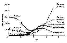
Fig. 1. Absorbance of yellow fluorescein in water solution at five wavelengths, as a function of pH, Ionic strength 0.10. Total concentration of fluorescein,  $2.407 \times 10^{-5} M$ .
