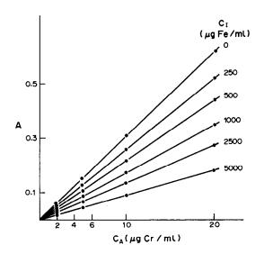
Fig. 3. Effect of iron on the calibration curve for chromium in the air-acetylene flame.
