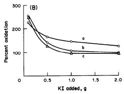
Fig. 1. Oxidation of 2-MBA by CAT, A, Effect of H<sub>2</sub>SO<sub>4</sub> concentration on oxidation of 2-MBA with (a) 0.10, (b) 0.50 and (c) 1.00 g of KI added. B, Effect of added KI on oxidation of 2-MBA at (a) 0.05, (b) 0.20 and (c) 0.35M H,SO<sub>4</sub> concentration.
