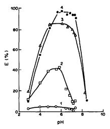
Fig. 2. Effect of pH on extraction of copper with alkyltrimethylammonium ions. The initial concentration of alkyltrimethylammonium ion in the aqueous phase is  $1 \times 10^{-3}M$ . 1, OTMA<sup>+</sup>; 2, DTMA<sup>+</sup>; 3, DDTMA<sup>+</sup>; 4, TDTMA<sup>+</sup>.
