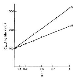
Fig. 10. Determination of molybdenum in the presence of vanadium (as vanadium chloride) in a graphite tube at 2800°. Test sample: 100 ng Mo/ml and 1 mg V/ml. Curve A: without buffer interferent;  $c_{\rm App_\infty} = 99$  ng/ml. Curve B: buffer interferent 5 mg (NH<sub>4</sub>)<sub>2</sub>HPO<sub>4</sub>/ml;  $c_{\rm App_\infty} = 99$  ng/ml.
