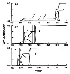
Fig. 15. Same as Fig. 14, but 5-ml injection. The yields obtained with the three columns are 0 (A), 0.15 (B) and 0.53 (C) for the first component, respectively. For the second component, they are 0 (A), 0.23 (B) and 0.83 (C) respectively.
