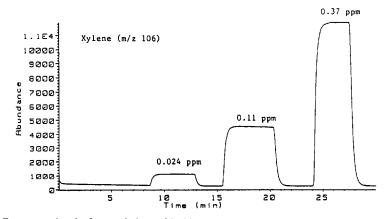
Fig. 16. Response signals for methylene chloride (m/z 84) and xylene (m/z 106) with interface B (Fig. 15) at 75°.
