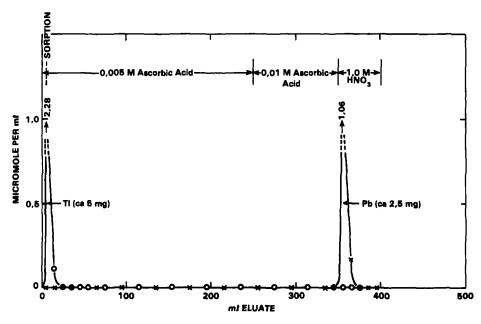
Fig. 2. Elution curve for Pb(II)-Tl(I): 0.5 ml of Chelex 100, H<sup>+</sup>-form, 100-200 mesh; column length 10 mm, diameter 8.0 mm; flow-rate 3.5 ± 0.3 ml/min.
