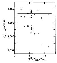
Fig. 4. Dependence (on indicator concentration) of the EDTA concentration obtained by the two methods for the zinc(II)-BT system.  $C_{\rm zn} = 1.700 \times 10^{-3} M$  at the equivalence-points.  $\bigcirc$ , calculated from the inflexion point;  $\triangle$ , calculated from the equivalence-point by equation (9).
