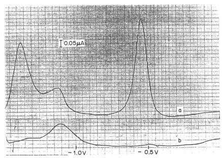
Fig. 4. Differential pulse polarograms of (a) nifedipine solution at pH 6 in ethanolic phosphate buffer (30:70 v/v) after irradiation with ultraviolet light for 24 hr, (b) ethanolic phosphate buffer (30:70 v/v), after irradiation as for (a).
