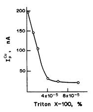
Fig. 7. Dependence of DP-AV peak current for  $4 \times 10^{-8} M$  Cu on Triton X-100 concentration. Supporting electrolyte: 0.1 M ammonia buffer,  $5 \times 10^{-4} M$  nioxime.  $t_{\rm acc} = 60$  sec;  $E_{\rm acc} = -0.2$  V.
