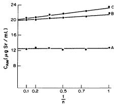
Fig. 11. Determination of strontium in the presence of aluminium in the air-acetylene flame. Test sample:  $20~\mu g$  Sr/ml and  $30~\mu g$  Al/ml. Curve A: without buffer interferent;  $c_{\text{App}_{\infty}} = 12.4~\mu g/\text{ml}$ . Curve B: buffer interferent 5 mg Al/ml;  $c_{\text{App}_{\infty}} = 20.3~\mu g/\text{ml}$ . Curve C: buffer interferent 5 mg La/ml;  $c_{\text{App}_{\infty}} = 19.8~\mu g/\text{ml}$ .
