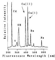
Fig. 6. A multielement analysis of a synthetic mixture of the five elements studied.
