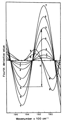
Fig. 6. Fourth-derivative spectra of  $MnO_4^-$  ion used for the calibration graph in the zero-crossing technique: 1-7, 0.25, 0.5, 1.0, 2.0, 3.0, 4.0 and 5.0  $\mu$ g/10 ml Mn; 8, 50 mg/ml Ni; 9, 80 mg/ml Ni.
