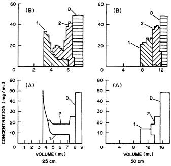
Fig. 16. Comparison between our simulated profiles (bottom) and the experimental results (top) previously published by Frenz. Displacement of a resorcinol/catechol mixture on two columns, one 25 cm long (left-hand two diagrams), the other 50 cm long (right-hand two diagrams), see text.
