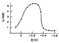
Fig. 4. Influence of accumulation potential on the peak stripping current. Nifedipine concentration  $5 \times 10^{-8} M$ . Other conditions as for Fig. 3.
