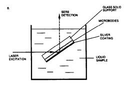
Fig. 3. Substrate for in situ analysis: (A) front surface SERS measurements; (B) back surface SERS measurements.
