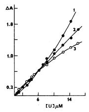
Fig. 1. Typical calibration plots for the system  $UO_2^{2+}$ -CAB-Septonex.  $c_L = 2 \times 10^{-5} M$ ,  $c_T = 6 \times 10^{-4} M$ , pH 5.6, I = 0.05, 5% v/v ethanol 1, 635 nm,  $\epsilon = 1.34 \times 10^5$  1. mole<sup>-1</sup>.cm<sup>-1</sup>; 2, 625 nm,  $\epsilon = 1.04 \times 10^5$  1. mole<sup>-1</sup>.cm<sup>-1</sup>; 3, 615 nm,  $\epsilon = 0.88 \times 10^5$  1. mole<sup>-1</sup>.cm<sup>-1</sup> ( $\epsilon$  calculated by regression analyses of the linear parts).
