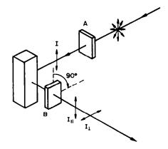
Fig. 2. Simplified representation of the fluorescence polarization process. A: excitation polarizer; B: emission polarizer; I: exciting polarized radiation;  $I_1$  and  $I_{\perp}$ : polarized fluorescence obtained with the two polarizers oriented in parallel and perpendicularly, repectively.
