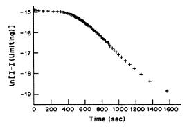
Fig. 8. Plot of  $\ln[I - I_{\rm L}]$  vs. time for the transient in Fig. 7. Slope = -0.00375, y-intercept = -13.28, square of the correlation coefficient = 0.9965,  $D_{\rm Non} = 1.4 \times 10^{-8}$  cm<sup>2</sup>/sec.
