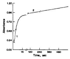
Fig. 2. Typical absorbance vs. time profile obtained in the analysis of a mixture of 1- and 2-naphthols (both  $25 \mu g/ml$ ) by the stopped-flow technique. I and 2 are the zones selected to measure  $V_1$  and  $V_2$ , respectively for short (data collection rate, 200 msec/point) and long (data collection rate, 1 sec/point) reaction times. Experimental conditions as described in procedure.
