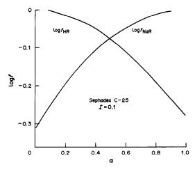
Fig. 3. Log  $f_{HR}$  and  $\log f_{NaR}$  obtained from equations (15) and (16) plotted against  $\alpha$  for Sephadex C-25 and  $I = 0.100M \text{ (Na)ClO}_4.$
