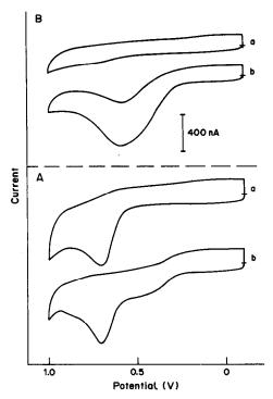
Fig. 2. Cyclic voltammetric response at the plain CoPC (A) and CoPC/Nafion (B) coated electrodes. (a) Response for  $2 \times 10^{-4}M$  oxalic acid; (b) as (a) but after addition of  $2 \times 10^{-4}M$  hydrazine. Supporting electrolyte, 0.05M phosphate buffer (pH 5.0); scan-rate 100 mV/sec.
