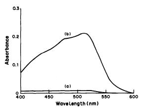
Fig. 1. Absorption spectra of iron(II)-phen-TPB complex and reagent blank in the eluent: (a) reagent blank; (b)  $11.2 \mu g$  of Fe(II), measured against (a).
