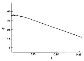
Fig. 4. Effect of ionic strength on the fluorescence intensity:  $C_{\rm Cd} = 8.90 \times 10^{-7} M$ ,  $C_{\rm L} = C_{\rm E} = 6.23 \times 10^{-6} M$ .  $I_{\rm F}$  in arbitrary units.
