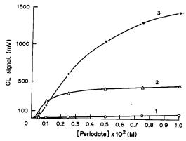
Fig. 5. Periodate calibration curves at a ratio of  $[Pg]_0/[Hx]_0 = 1$ . Conditions: pH 8.0;  $[Hx]_0$  1.0 × 10<sup>-4</sup>M (1), 5.0 × 10<sup>-4</sup>M (2), 1.0 × 10<sup>-3</sup>M (3).
