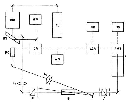
Fig. 1. Experimental system for atomic polarization spectroscopy. Solid lines indicate optical paths and broken lines show electrical connections. A, analyzer prism; AL, argon-ion laser; B, slot burner; BS, beam splitter; CR, chart recorder; DR, high-voltage driver; F, line filter; HV, power supply; L<sub>1</sub> and L<sub>2</sub>, focusing lenses; LIA, lock-in amplifier; P, polarizer prism; PMT, photomultiplier tube; RDL, ring dye laser; WG, waveform generator; WM, wavemeter.
