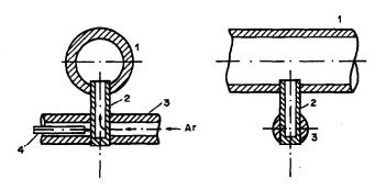
Fig. 2. Scheme of combined atomization equipment (CAE): 1, atomization tube; 2, carbon "beaker-rod"; 3, rods for heating the beaker-rod; 4, thermocouple.
