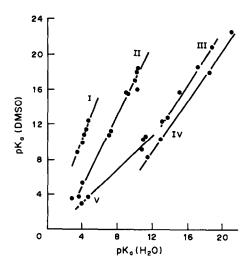
Fig. 4. Plot of pK<sub>a(DMSO)</sub> against pK<sub>a(H2O)</sub> for 25 HA and 5 BH<sup>+</sup> acids. Lines: I—carboxylic acids, II—phenols, III—nitroanilines, IV—CH-acids, V—ammonium acids (BH<sup>+</sup>).
