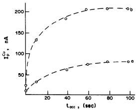
Fig. 5. Dependence of DP-AV peak current for  $1.5\times 10^{-8}M$  Cu (a) and  $4\times 10^{-8}M$  Cu (b) in 0.1M ammonia buffer containing  $5\times 10^{-4}M$  nioxime, on the preconcentration time in stirred solution.  $E_{\rm acc}=-0.2$  V.
