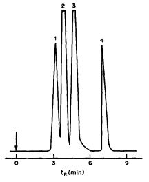
Fig. 1. Chromatogram of model mixture of benzene (1) and monosubstituted phenols: o-nitrophenol (2), o-chlorophenol (3), o-cresol (4). Column Silasorb 600,  $10 \mu m$ ,  $200 \times 6 mm$ ; mobile phase 2.5 v/v butan-1-ol in n-hexane; 25°C; spectrophotometric detector (254 nm).
