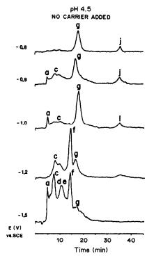
Fig. 5. HPLC of "no carrier added" <sup>99m</sup>Tc-HEDP mixtures prepared by coulometric reduction of <sup>99m</sup>TcO<sub>4</sub><sup>-</sup> at various reduction potentials. Conditions: Gamma-ray detection at 140 keV, 0.2 ml/min flow-rate, ambient temperature.
