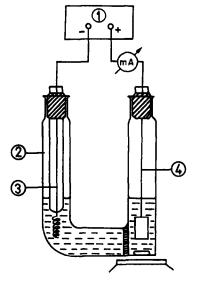
Fig. 1. Schematic diagram of the apparatus for coulometric titration of bases with visual end-point detection: 1, voltage-current stabilizer; 2, electrolytic cell; 3, Pt cathode; 4, H<sub>2</sub>/Pd anode.
