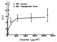
Fig. 5. Bleaching of Rhodamine B by Cl₂ in the gas phase. Comparisons of two different methods: means and error bars for Rhodamine B aerosol (♠); filter impregnated with Rhodamine B (○).
