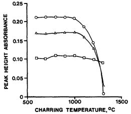
Fig. 1. Effect of ashing temperature on the peak-height absorbance of 25  $\mu$ g/l. tin:  $\bigcirc$ , 5 g/l.  $(NH_4)_2HPO_4 + 0.5$  g/l.  $Mg(NO_3)_2 + 0.2\%$  v/v HNO<sub>3</sub> (modifier A);  $\triangle$ , 2 g/l.  $(NH_4)_2HPO_4 + 0.4$  g/l.  $(NH_4)_2Cr_2O_7 + 2\%$  v/v HNO<sub>3</sub> (modifier B);  $\square$ , 50 g/l. ascorbic acid + 0.2 g/l. Fe (as ferric nitrate) (modifier C).
