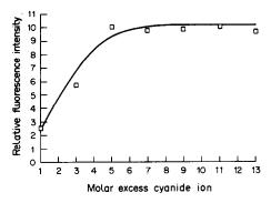
Fig. 4. Fluorescence intensity vs. molar excess of cyanide.
