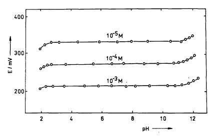
Fig. 2. Electrode response as a function of pH for different nitrate activities.
