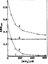
Fig. 5. Effect of CT concentration on extent of interference by ammonia. Curve (1) [CT] =  $38.6\mu M$ , [Br] =  $0\mu M$ ; (2) [CT] =  $38.6\mu M$ , [Br] =  $25\mu M$ ; (3) [CT] =  $386\mu M$ , [Br] =  $0\mu M$ ; (4) [CT] =  $386\mu M$ , [Br] =  $25\mu M$ .
