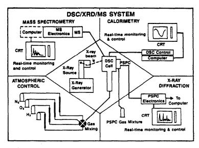
Fig. 22. Schematic diagram of the DSC/XRD/MS instrument. PSPC, position-sensitive proportional counter.
