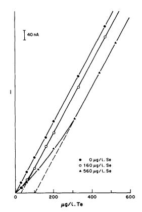
Fig. 2. Calibration curves for tellurium in presence of different fixed amounts of selenium.
