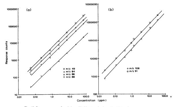
Fig. 17. Response curves of methylene chloride (a) and xylene (b) with interface B (Fig. 15).
