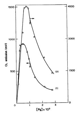
Fig. 2. Effect of pyrogallol concentration at  $[Hx]_0 = 1.0 \times 10^{-3} M$ . Conditions: pH 8.0;  $[IO_4^-]_0$   $1.0 \times 10^{-3} M$  (1),  $1.0 \times 10^{-2} M$  (2).
