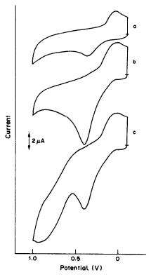
Fig. 3. Cyclic voltammetric response of the CoPC/Nafion (75/25% v/v) coated electrode. (a) Response for  $5 \times 10^{-5} M$  dopamine, (b) as (a) but following 5 min accumulation (with 400 rpm stirring at open-circuit), (c) as for (b) but after addition of  $2 \times 10^{-3} M$  hydrogen peroxide. Scan-rate and electrolyte as for Fig. 1.
