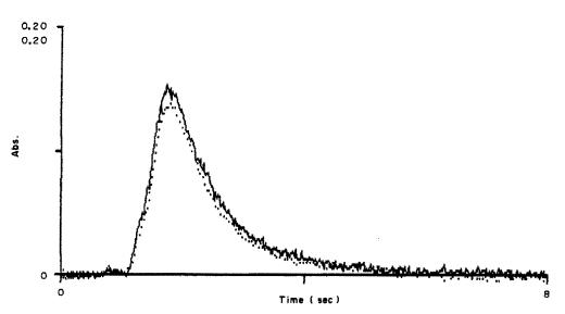
Fig. 3. Typical absorbance profile for Cu for the conditions of this test.
