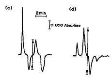
Fig. 2. Types of recordings obtained for different sample and standard concentrations: (a) and (b) normal x-t recordings; (c) and (d) derivative recordings and measuring procedure. Concentrations: (a) and (c) standard 1  $\mu$ g/ml formaldehyde, sample 1  $\mu$ g/ml formaldehyde; (b) and (d) standard 1  $\mu$ g/ml formaldehyde, sample 4  $\mu$ g/ml formaldehyde.
