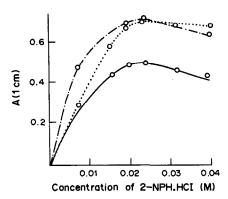
Fig. 2. Influence of 2-NPH·HCl concentration on the colour intensity developed from: 1  $\mu$ mole of penicillin G sodium (-----); 2  $\mu$ mole of ampicillin (....); 3  $\mu$ mole of cephalexin sodium (-----).
