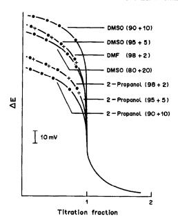
Fig. 3. Effect of various solvents on the titration endpoint break in the determination of 0.05 mmole of  $CO_2$ .  $C_{MEA} = 1\%$ . Points—experimental; solid lines—calculated for MEAH<sup>+</sup> in the presence of an excess of MEA.
