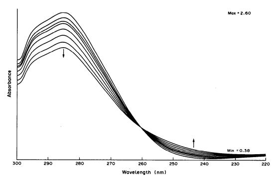
Fig. 6. Time-dependent spectra of an aqueous chlorimine solution at pH 10. Multiple spectra are recorded over a 4-hr interval. The absorption band of chlorimine at 287 nm decreases with time, owing to hydrolysis.
