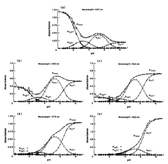
Fig. 3. Absorbance vs. pH curves for the four prototropic forms of yellow fluorescein at five wavelengths (a)—(e). For each wavelength and at each pH the four component absorbances sum to the observed absorbance. Symbols are the same on all five graphs. Total A, original data  $\bigcirc$ ;  $A_{H_3F_1} \triangle$ ;  $A_{H_2F_1} + A_{HF_1}$   $\times$ ;  $A_{F_1} \blacksquare$ .
