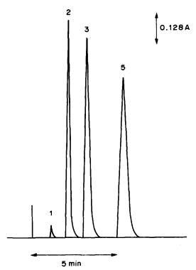
Fig. 2. Effect of flow change-over time: 1, 1 min; 2, 2 min; 3, 3 min; 5, 5 min. Reagent solution, Glucose test C Wako, 0.2 ml/min; carrier, 0.2M NaH<sub>2</sub>PO<sub>4</sub>/Na<sub>2</sub>HPO<sub>4</sub>, pH 7.4, flow-rate 1 ml/min; sample, glucose, 0.200 g/l., sample volume about 3 μl.
