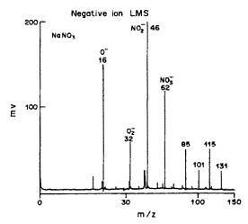
Fig. 3. Negative-ion laser mass spectrum of NaNO3.
