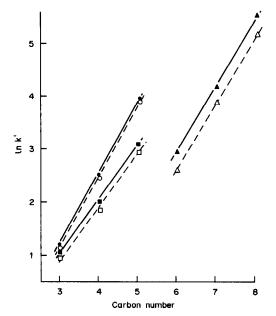
Fig. 2. Plots of  $\ln k'$  vs. carbon number, showing changes in retention with addition of methylene groups. Solid line and filled symbols: data obtained before surface reordering/resolvation. Dashed line and open symbols: data obtained after surface reordering/resolvation.  $\bullet$ ,  $\bigcirc$ : propanol, butanol, pentanol.  $\blacktriangle$ ,  $\triangle$ : phenol, p-methylphenol, p-ethylphenol.  $\blacksquare$ ,  $\square$ : 2-propanol, tert-butyl alcohol, tert-pentyl alcohol.
