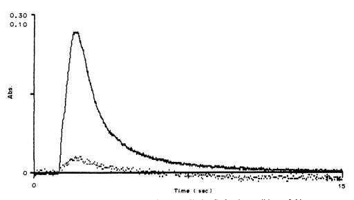
Fig. 1. Typical absorbance profile for Cr for the conditions of this test.
