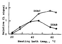
Fig. 2. Effect of reaction temperature on the CL signal for sulphide. R<sub>1</sub>:  $1 \times 10^{-4}M$  TCNQ/40% CH<sub>3</sub>CN; R<sub>2</sub>:  $1 \times 10^{-3}M$  DDAB (DOAC)/ $1 \times 10^{-2}M$  NaOH; [S<sup>2-</sup>]:  $3 \times 10^{-4}M$ ; flow-rate: 6 ml/min.
