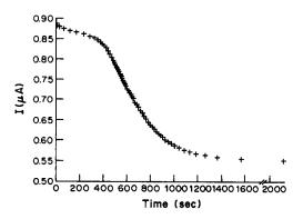
Fig. 7. Current-time transient of a 2.79mM nonactin membrane in 0.001M NH<sub>4</sub>Cl. Bias is -2.33 V.
