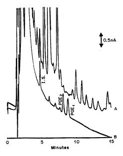
Fig. 5. Chromatograms of urinary prostaglandins derivatized with PNBA. Chromatographic conditions: column, Supelcosil LC-8-DB, 15 cm × 4.6 mm; mobile phase, acetonitrile/50mM sodium acetate, pH 6 (50/50); flow, 1 ml/min. (A) Extracted and derivatized human urine sample. (B) Prostaglandins E<sub>1</sub> and E<sub>2</sub> with internal standard (I.S.) cyclopentanone.
