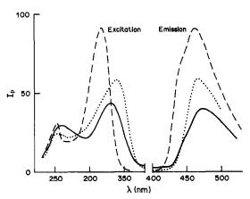
Fig. 2. Effect of pH on the excitation and emission RTP spectra of 6-mercaptopurine (10<sup>-3</sup>M) on W-40 filter paper, in the presence of 1M KI: · · · · neutral solution (sensitivity × 1); — acidic solution (sensitivity × 4); ---- basic (1M NaOH) (sensitivity × 1).
