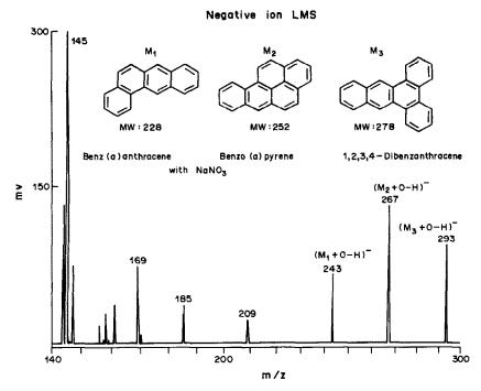
Fig. 7. Negative-ion laser mass spectrum of a mixture of benz(a)anthracene, benz(a)pyrene, and 1,2,3,4-dibenzanthracene, mixed with NaNO<sub>3</sub>.
