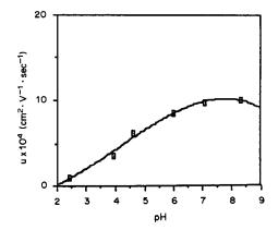
Fig. 6. Effect of pH of  $10^{-2}M$  phosphate buffers on electro-osmotic flow coefficients in untreated fused-silica capillaries.
