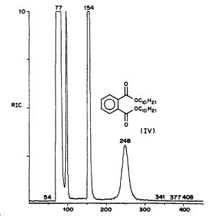
Fig. 3. LC/MS total ion chromatogram of an extract from an unknown polymer: column, 25 cm × 4.6 mm Zorbax ODS; eluent, 100% CH<sub>3</sub>OH 1 ml/min; discharge ionization 1.4 kV.
