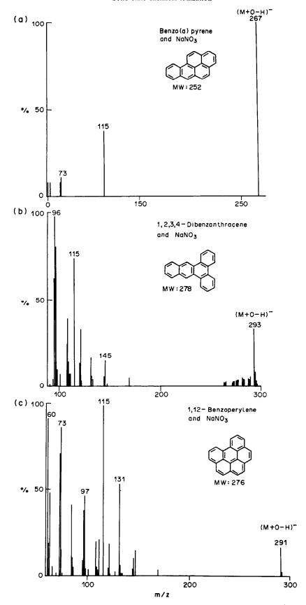
Fig. 4. Negative-ion LMS of (a) benzo(a)pyrene, (b) 1,2,3,4-dibenzanthracene, (c) 1,12-benzoperylene, mixed with sodium nitrate.
