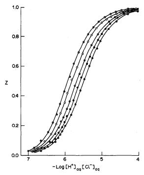
Fig. 1. Experimental degree of neutralization of the amine, Z, as a function of  $-\log[H^+]_{aq}[Cl^-]_{aq}$  for various concentrations of Amberlite LA-1 in 1,2-dichloroethane: 0.015M  $\Phi$ ; 0.026M  $\Phi$ ; 0.043M  $\Phi$ ; 0.083M  $\bigcirc$ ; 0.173M  $\Phi$ , lines were calculated with  $\log R_{11} = 5.28$  and  $\log R_{22} = 12.50$ ;  $[Cl^-] = 1M$ .
