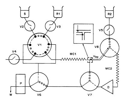
Fig. 5. ACCAS sequential reaction system. V1: 6-port rotary valve; V2-V5 on/off valves; V6-V8: 3-way valves; other symbols as in Fig. 1. Inset shows location of Pt-probes in the tee.
