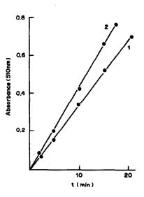
Fig. 5. Influence of irradiation time on yield of Fe(II)-(phen), for acriflavine: (1) open to atmosphere; (2) in absence of oxygen; pH 5.7,  $2 \times 10^{-2}M$  EDTA,  $1 \times 10^{-3}M$  MV<sup>2+</sup>,  $4 \times 10^{-3}M$  phen,  $2\mu M$  acriflavine.
