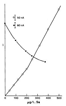
Fig. 1. Calibration graph for selenium ( $\bigcirc$ ) in presence of a fixed concentration of tellurium (80  $\mu$ g/l.) and trend of the tellurium signal ( $\bigcirc$ ).
