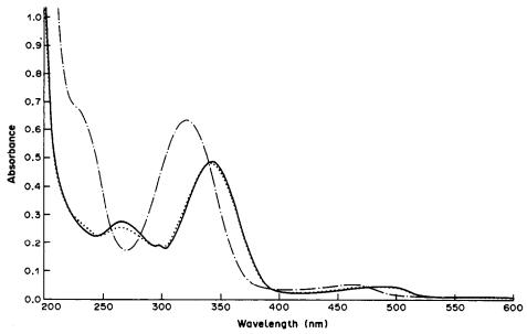
Fig. 2. Absorption spectra of the protonated (—— and ···) and deprotonated (—·—) NBD ring-substituted crown ether.
