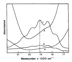
Fig. 1. Absorption spectra of MnO<sub>4</sub><sup>-</sup> and Ni<sup>2+</sup> ions in 0.2M H<sub>2</sub>SO<sub>4</sub>: 1, 2.5  $\mu$ g/ml Mn; 2, 0.5  $\mu$ g/ml Mn; 3, 25 mg/ml Ni; 4, 5 mg/ml Ni.
