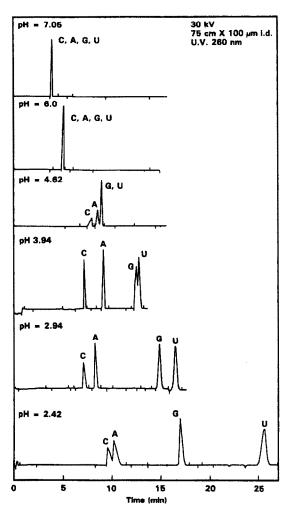
Fig. 7. Effect of buffer pH on the CZE separation of nucleosides in a short 75 cm  $\times$  100  $\mu$ m i.d. capillary with UV detection at 260 nm: cytidine (C), adenosine (A), guanosine (G), and uridine (U).
