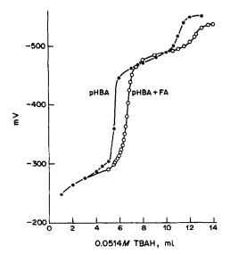
Fig. 2. Non-aqueous titrations of pHBA in the presence and absence of Bersbo fulvic acid: ● 38.53 mg of pHBA; ○ 38.53 mg of pHBA + 13.3 mg of Bersbo FA.
