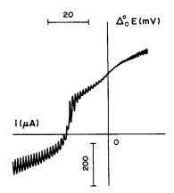
Fig. 3. Polarogram of the chelate La-HTTA. Aqueous phase: 0.2M NaOAc, 0.3mM La, pH  $7.0 \pm 0.1$ . DCE phase: 0.01M THA·TPB, 4mM HTTA.
