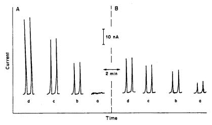
Fig. 7. Flow-injection peaks for oxalic acid solutions containing increasing hydrogen peroxide concentrations, at the CoPC/Nafion (84/16% v/v) (A) and CoPC (B) coated electrodes:  $1 \times 10^{-4} M$  oxalic acid; (b-d), as for (a) but after successive additions of  $2 \times 10^{-4} M$  hydrogen peroxide. Applied potential, +0.80 V; other conditions as for Fig. 6.
