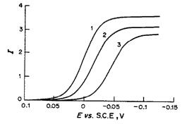
Fig. 2. Curves of current intensity (in arbitrary units) vs. potential for the system Cd–Cl, calculated by equation (11): 1,  $[Cl^-] = 5.93 \times 10^{-6} M$ ; 2,  $[Cl^-] = 2.00 \times 10^{-4} M$ ; 3,  $[Cl^-] = 9.51 \times 10^{-4} M$ . Constants  $K_1 = 21.33$ ,  $K_2 = 2.55$  and  $K_3 = 0.60$  were taken from Leggett.<sup>3</sup>
