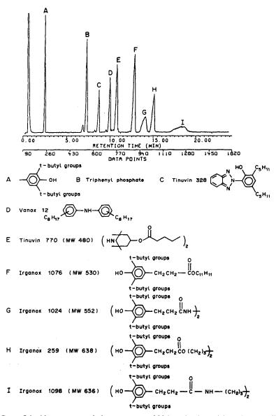
Fig. 10. Gram-Schmidt reconstructed chromatogram of high molecular-weight polymer additive standards analyzed by GC/FT-IR with a 1-m capillary column and high lightpipe interface temperatures.
