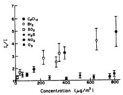
Fig. 6. Bleaching of Rhodamine B aerosol: interference by various trace gases, relative humidity 85%; means and error bars.
