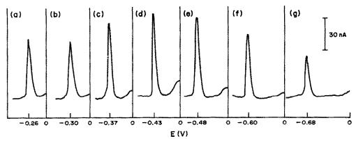
Fig. 5. Influence of pH on the voltamperogram peak current. Britton-Robinson buffer, 0.25M in NaClO<sub>4</sub>. Nifedipine concentration 5 × 10<sup>-8</sup>M. pH: a 1.48; b, 2.10; c, 3.05; d, 4.44; e, 5.60; f, 7.83; g, 9.70.
