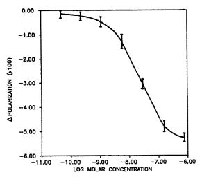
Fig. 6. Calibration curve for bovine insulin, with Ag\*F  $(5.2 \times 10^{-10} M)$  and Ab  $(1.7 \times 10^4$  dilution) in pH 7.6 TRIZMA buffer with 0.025M NaSy.
