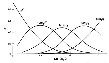
Fig. 2. Fraction of indium(III) in its various forms, as a function of free azide ion concentration.
