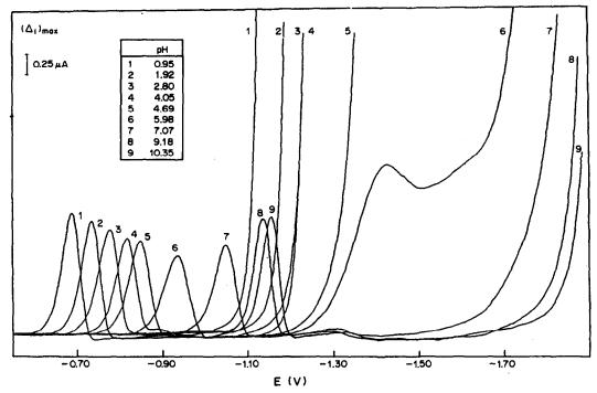
Fig. 4. DPP polarograms of clotiazepam at different pH values.
