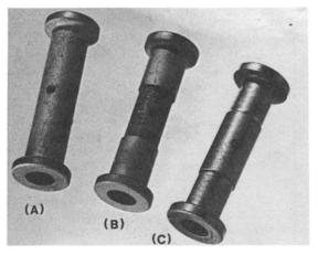
Fig 1 SP-9 atomizer tube designs; (A) unmodified tube, (B) modified tube I, (C) modified tube II
