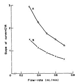
Fig. 2. Detector response as a function of flow-rate: A—hydrogen peroxide injection; B—glucose injection into enzyme reactor (peroxide detection), glucose and hydrogen peroxide concentrations were equal.
