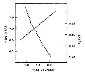
Fig. 2. Dependence of the logarithm of the peak current ( $\bullet$ ) and peak potential ( $\triangle$ ) on the logarithm of the potential scan-rate. Nifedipine concentration:  $10^{-6}M$ .
