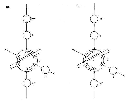
Fig. 1. Schematic flow diagrams: (a) 1st position, (b) 2nd position; RP, reagent solution pump; I, injector; L, reaction loop; V, 6-way valve; CP, carrier pump; D, detector.
