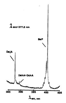
Fig. 3. Fluorescence spectrum of four-component dibenzacridine mixture in solid argon (at 15 K) at the optimum excitation wavelength for dibenz[a, j]acridine.
