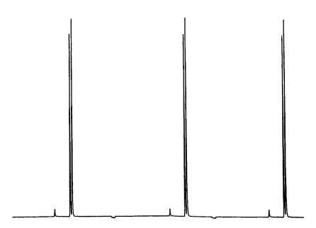
Fig. 4. Example of injection-to-injection reproducibility obtained with automated electromigration injection.
