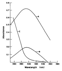
Fig. 1. Absorption spectra: A, Ti-HDPBA-SCN<sup>-</sup>; B, Ti-HDPBA; C, reagent blank.
