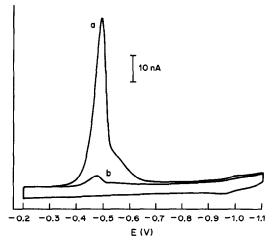
Fig. 1. (a) Repetitive cyclic voltamperograms for  $10^{-6}M$  nifedipine in Britton-Robinson buffer (pH 4.4), after stirring for 60 sec at -0.2 V. (b) An analogous voltamperogram without accumulation. Scan-rate 30 mV/sec.
