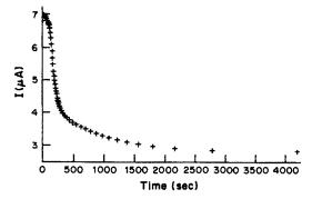
Fig. 9. Current-time decay of a 5.39mM TDA membrane. Bias is -18 V.
