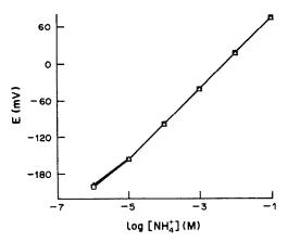
Fig. 3. Potentiometric ammonium response of various cellulose triacetate-based membranes doped with nonactin: (△) hydroxylated asymmetric membrane; (×) aminated asymmetric membrane; (□) unmodified cellulose triacetate membrane.
