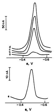
Fig. 3. DP-AV curves (a-d) and DC-AV curve (e) for  $4 \times 10^{-8}M$  Cu in 0.1M ammonia buffer,  $5 \times 10^{-4}M$  nioxime, obtained in unstirred (a, c) or stirred (b, d, e) solution. Preconcentration period: (a) 0; (b) 20; (c) 320; (d, e) 60 sec: preconcentration potential -0.2 V; scan-rate 26.3 mV/sec.
