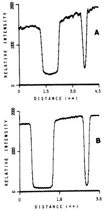
Fig. 2. Responses of the image dissector (A) and the photodiode array (B) to a test image.
