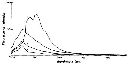
Fig. 4. Effect of varying concentration on the fluorescence emission spectrum of BAC: (a)  $1.78 \times 10^{-3}M$ ; (b)  $2.66 \times 10^{-3}M$ ; (c)  $4.03 \times 10^{-3}M$ ; (d)  $2.37 \times 10^{-2}M$ .
