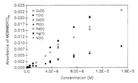
Fig. 2. Calibration graphs for nickel(II), mercury(II), cobalt(II), copper(II), iron(II), platinum(II), palladium(II) and thallium(III). All values were obtained by using the Radial Compression Cartridge column under the conditions described in the text.
