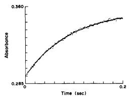
Fig. 1. Fit of a nonlinear reaction model (solid line) to absorbance data collected for the reaction of  $6.50 \times 10^{-3} M$  Cl<sub>T</sub> with  $1.5 \times 10^{-4} M$  N<sub>T</sub>. Solution absorbance data collected at 245 nm for the appearance of NH<sub>2</sub>Cl. Reaction model is based on a reaction order of 1.0 for NH<sub>3</sub>.
