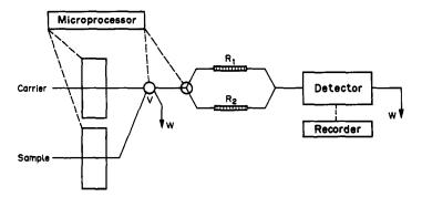
Fig. 4. Manifold with selecting valve for column replacement or regeneration without disrupting the monitoring process.
