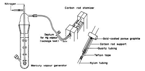
Fig. 1. Apparatus for the determination of mercury by cold vapour generation.
