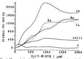
Fig. 4. The variation in fluorescence signal-to-noise ratio for each element as a function of spectrometer slit-width.
