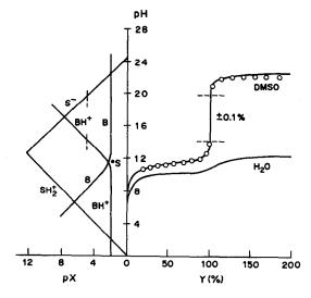
Fig. 8. Theoretical titration curves of atropine sulphate in DMSO/water mixture and in water (full lines). The experimental data are shown with open circles.
