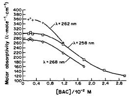
Fig. 3. Change in molar absorptivity of BAC with concentration.
