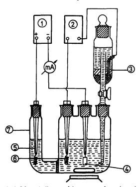
Fig. 2. Schematic diagram of the apparatus for coulometric titration of bases with potentiometric end-point detection: 1, voltage-current stabilizer; 2, pH meter; 3, mercury(I) acetate electrode; 4, H<sub>2</sub>/Pd anode; 5, Pt cathode; 6, H<sub>2</sub>/Pd indicator electrode; 7, electrolytic cell.
