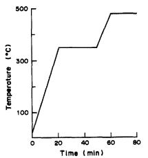
Fig. 1. Temperature programme for the decomposition of seaweed by fusion with sodium hydroxide.
