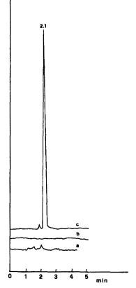
Fig. 1. Chromatograms of (a) a non-dialysed urine; (b) the same urine after dialysis; (c) a 50 mg/l. solution of ethanol in dialysed urine.
