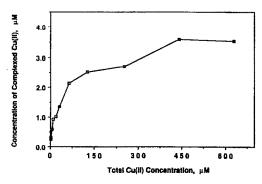
Fig. 6. Corrected titration curve for the Willamette River water sample.
