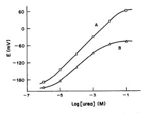
Fig. 6. Typical calibration curves for the urea electrodes prepared by using asymmetic ammonium-selective cellulose triacetate membranes: (A) urease-aminated membrane prepared by the one-step glutaraldehyde method; (B) urease-hydroxylated membrane prepared by the direct CDI activation method.
