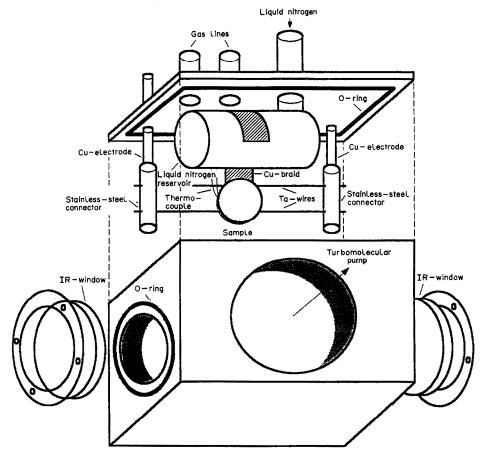
Fig. 3. High-vacuum cell for reflection-absorption FT-IR spectroscopy of adsorbates on single crystals.
