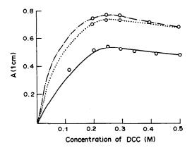
Fig. 3. Influence of DCC concentration on the colour intensity developed from: 1  $\mu$ mole of penicillin G sodium (----); 2  $\mu$ mole of ampicillin (....); 3  $\mu$ mole of cephalexin sodium (----).
