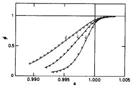
Fig. 3. Photometric titration curves for zinc(II).  $\Box$ ,  $C_{BT}/C_{Zn} = 3.39 \times 10^{-3}$ ;  $\triangle$ ,  $C_{BT}/C_{Zn} = 6.77 \times 10^{-3}$ ;  $\bigcirc$ ,  $C_{BT}/C_{Zn} = 1.129 \times 10^{-2}$ .  $C_{Zn} = 1.700 \times 10^{-3} M$  at the equivalence-points.
