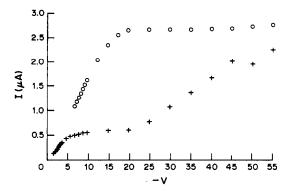
Fig. 3. Current-voltage curves for different nonactin concentrations in the membrane (sweep in the direction of increasing voltages): O, 14.8mM nonactin; +, 2.79mM nonactin.
