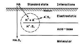
Fig. 1. Schematic presentation of the interactions in the Izmailov concept. The part encircled with a dashed line shows the Brønsted concept.
