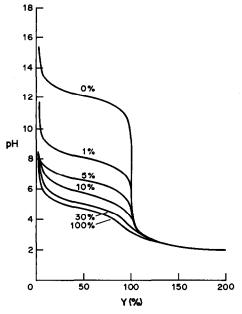
Fig. 3. Titration curves of amidopyrine in acetonitrile with increasing water content.
