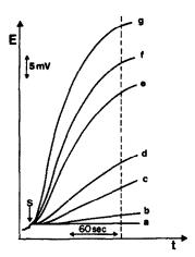
Fig. 3. Typical reaction curves of the FDNB-isoniazid reaction for calculation of the kinetic parameters and calibration graphs, at 25° and pH 9.0. [FDNB] =  $1.78 \times 10^{-3} M$ ; [isoniazid] (a) blank, (b)  $6.67 \times 10^{-5} M$ , (c)  $3.33 \times 10^{-4} M$ , (d)  $6.67 \times 10^{-4} M$ , (e)  $2.00 \times 10^{-3} M$ , (f)  $3.33 \times 10^{-3} M$ , (g)  $6.67 \times 10^{-3} M$ . Dashed line shows the  $\Delta E$  measurement in the fixed-time method.
