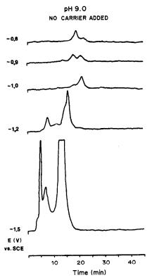
Fig. 9. HPLC of "no carrier added" 99mTc-HEDP mixtures prepared by coulometric reduction of TcO<sub>4</sub> at pH 9.0 and various reduction potentials. Conditions as for Fig. 5.
