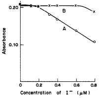
Fig. 3. The effect of choride on the calibration curve. The concentration of chloride was 0.01M in curve A, and 0.15M in curve B. The concentrations of Hg(II) and Sn(II) were 0.04µM and 4.4mM, respectively.
