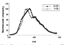
Fig. 5. Time-resolved emission spectra of pyrene:CD complexes in the presence of sec-butyl alcohol.
