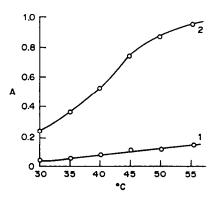
Fig. 6. Dependence of the reaction rate on temperature. (1) Uncatalysed reaction; (2) catalysed reaction; 1.0  $\mu$ g of Fe(III) per 25 ml.
