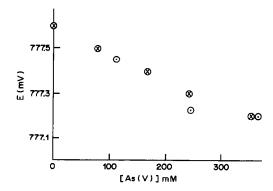
Fig. 3. Emf of cell (4) vs. arsenic acid concentration. Test solution: 5M hydrochloric acid. Ordinates: emf of the cell, mV. Abscissae: total concentration of arsenic(V), mM. ⊗ Addition of arsenic(V) to 5M HCl. ⊙ Dilution of concentrated arsenic(V) solution with 5M HCl.
