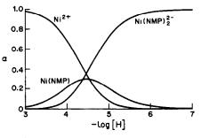
Fig. 5. Distribution of Ni(II) species in the Ni(II)-NMP system as a function of pH.  $C_L = 5 \times 10^{-5} M$ ,  $C_M = 1 \times 10^{-5} M$ .
