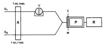
Fig. 1. Manifold and instruments used for the mixing and for monitoring the generated CL emission. (S1) carrier stream; (S2) reagent stream; (V) sample valve; (W) waste; (C) cell; (A) pump; (P) photomultiplier; (R) recorder.
