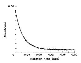
Fig. 3. Fit of a second-order reaction model (solid line) to absorbance data collected for the reaction of  $1.98 \times 10^{-3} M$  Cl<sub>T</sub> with  $5.11 \times 10^{-3} M$  N<sub>T</sub>. Solution absorbance data collected for the disappearance of OCl<sup>-</sup> at 292 nm.  $k' = 1.744 \times 10^4$ . Rate constant:  $k_1 = (3.24 \pm 0.05) \times 10^6$  1. mole<sup>-1</sup>. sec<sup>-1</sup>.
