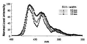
Fig. 2. Perylene TR emission spectra as a function of emission monochromator slit-width.
