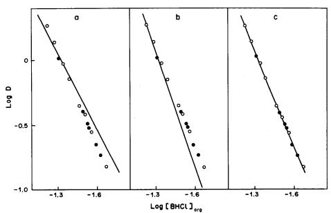
Fig. 4. Distribution ratio  $\log D$  vs.  $\log [BHCl]_{org}$ . Lines were calculated by using equation (14) for: (a) p=2; (b) p=3; (c) p=2 and p=3 (Table 2, model I).
