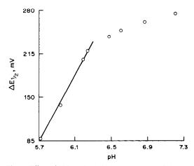
Fig. 4. Effect of pH on the half-wave potential of the wave from the La-HTTA chelate. Aqueous phase: 0.2M NaOAc, 0.2mM La, pH  $7.0 \pm 0.1$ . DCE phase: 0.01M THA TPB, 4mM HTTA.
