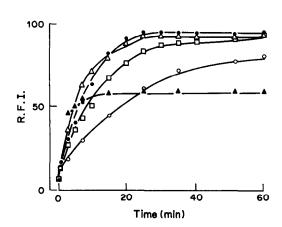
Fig. 5. Effects of reaction time and temperature with DMPD reaction on the fluorescence intensity: caffeine taken, 1.0 μg; ○, 30°; □, 40°; ●, 50°; △, 60°; ▲, 80°.
