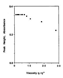
Fig. 8. Peak height vs. relative viscosity in two-line FIA (blank system). Peaks are for 2mM NaCl.
