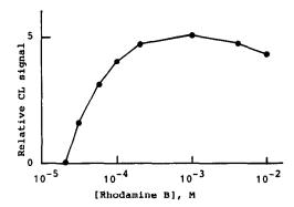
Fig. 3. Effect of Rhodamine B concentration on the signal for sulphide.  $[S^{2-}]1 \times 10^{-6}M$ . Other conditions as for Fig. 2 (DOAC system).
