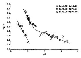
Fig. 4. The variation of the distribution coefficient (D) of Eu(III) in the presence of fulvic acid, as a function of pH and ionic strength.
