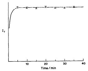
Fig. 3. Rate of production of fluorescence for 3.6 ppm carbaryl in presence of 6% Nemol K-1030 at pH 12.
