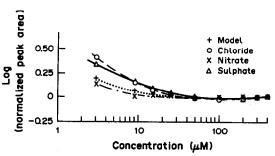
Fig. 2. Log-log plots of normalized peak area vs. concentration for calibrations in Fig. 1 and the model in Fig. 5.
