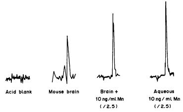
Fig. 7. ZETA-LEAFS furnace signals for the determination of Mn in mouse brain tissue.
