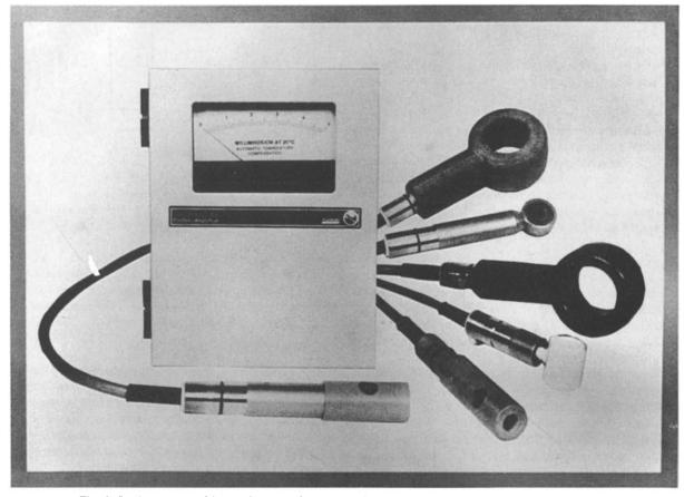
Fig. 3. Various types of immersion cells for electrodeless conductivity with an associated instrument (courtesy of The Foxboro Company).
