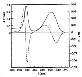
Fig. 1. Absorption curve of 0.001% salicylic acid solution (——) first-derivative D<sub>1</sub> curve (———).
