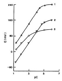
Fig. 1. Calibration curves. Oxacillin-CTOP electrode (1), oxacillin-CTOA electrode (2), oxacillin-CTOAs electrode (3).
