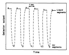
Fig. 9. High-speed chart record of an ACCAS output for 1800 samples/hr. The dashed lines indicate pen transitions from one segment to another; the speed of this transition is too high for a consistently legible record. Note that the passage of the interface through the detection zone results in a spike before either segment.
