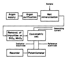
Fig. 1. Block diagram of the measuring set-up.
