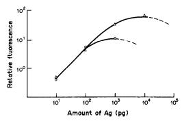
Fig. 4. The upper range of the ZETA-LEAFS calibration curves for Ag (○) measured with laser tuned to the resonance wavelength (328.1 nm), and (△) with laser tuned 9 pm away from the resonance wavelength.
