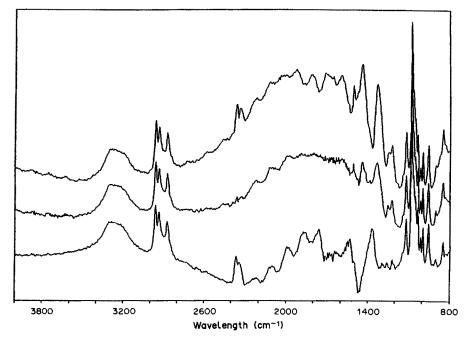
Fig. 7. Three successive dual-beam spectra of 5 monolayers of n-butanol (100 scans each, mirror velocity 1.266 cm/sec, resolution 4 cm<sup>-1</sup>).
