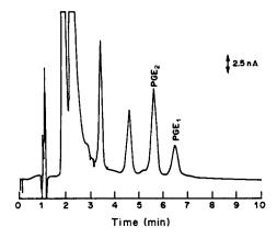
Fig. 3. Chromatogram of DNPH derivatives of prostaglandins extracted from spiked plasma sample. Chromatographic conditions: column, Supelcosil LC-8-DB,  $15 \text{ cm} \times 4.6 \text{ mm}$ ; mobile phase, acetonitrile/50mM sodium acetate, pH 4 (65/35); flow, 1 ml/min; detection, -0.90 V.
