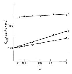
Fig. 12. Determination of platinum in the presence of vanadium in the air-acetylene flame. Test sample:  $100~\mu g$  Pt/ml and 3 mg V/ml. Curve A: without buffer interferent;  $c_{\rm App_\infty} = 170~\mu g/\rm ml$ . Curve B: buffer interferent 5 mg Pd/ml;  $c_{\rm App_\infty} = 100~\mu g/\rm ml$ . Curve C: buffer interferent 5 mg La/ml;  $c_{\rm App_\infty} = 100~\mu g/\rm ml$ .
