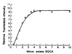
Fig. 3. Fluorescence intensity vs. molar excess of BQCA.
