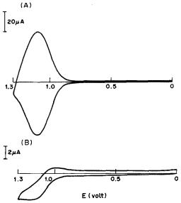
Fig. 9. Cyclic voltamperograms for a polymer-modified glassy-carbon electrode before (A) and after 4 hr (B) use as an NO<sub>2</sub> detector. Coating was performed with 122 cycles. Scan-rate 50 mV/sec. Supporting electrolyte 0.10M KCl (pH 4.00).
