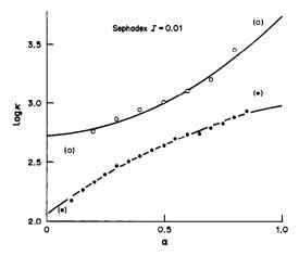
Fig. 2. Log  $\kappa$  plotted against  $\alpha$  for the system H<sup>+</sup>-Na<sup>+</sup> on Sephadex at 298.2 K. The ionic strength in the aqueous phase I = 0.010M (Na)ClO<sub>4</sub>.  $\bigcirc$  Sephadex C-25; ● Sephadex C-50. The curves were calculated from equation (5) with the parameters in Table 5. The experimental points excluded from calculation are given in parentheses.
