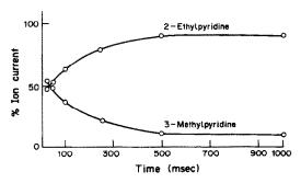
Fig. 1. Attainment of equilibrium for a mixture of 2-ethylpyridine and 3-methylpyridine in an ion trap. The relative basicities of the two bases is calculated as 8.6 kJ/mole from the concentration ratio of protonated 2-ethylpyridine to protonated 3-methylpyridine.
