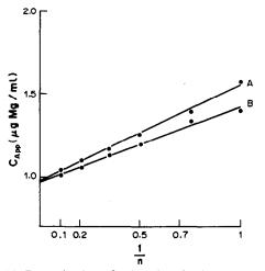
Fig. 14. Determination of magnesium in the presence of aluminium, titanium and calcium in the air-acetylene flame. Test sample: 1  $\mu$ g Mg/ml, 3 mg Al/ml, 3 mg Ti/ml and 3 mg Ca/ml. Curve A: without buffer interferent;  $c_{\rm App_{\infty}} = 0.97$   $\mu$ g/ml. Curve B: buffer interferent 5 mg La/ml;  $c_{\rm App_{\infty}} = 0.96$   $\mu$ g/ml.
