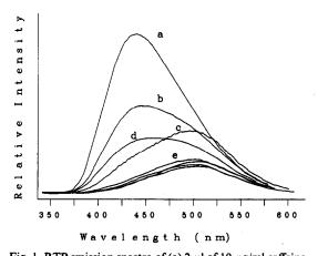
Fig. 1. RTP emission spectra of (a)  $2 \mu l$  of  $10 \mu g/ml$  caffeine, (b)  $2 \mu l$  of  $5 \mu g/ml$  caffeine, (c)  $2 \mu l$  of  $10 \mu g/ml$  theophylline, (d) mixture of  $2 \mu l$  containing 5 ppm caffeine, 5 ppm theophylline; (e) blanks for (a)–(d) on Whatman No. 1 paper prepared with  $3 \mu l$  of 0.1M NaOH and  $3 \mu l$  of 1M KI. Similar spectra occur on Whatman DE-81 under the same conditions. Excitation and emission wavelengths 275 and 440 nm, respectively.
