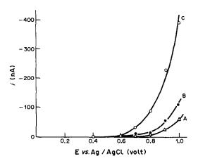
Fig. 3. Voltamperogram showing the response to NO<sub>2</sub> (30 ppb v/v) at a modified (10% w/w) carbon paste electrode. Flow-rate 2.0 ml/min, injected sample size: 250 μl. Carrier supporting electrolyte: 0.10M KCl (pH 4.00). (A) Response to air injection for both chemically modified and unmodified electrodes; (B) NO<sub>2</sub> response of an unmodified carbon paste electrode; (C) NO<sub>2</sub> response of modified carbon paste electrode.
