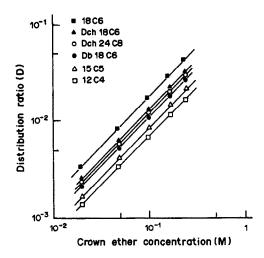
Fig. 2. Effect of crown ether concentration in chloroform on the extraction of Co(II) from perchlorate aqueous medium at constant ionic strength 0.1 (H<sup>+</sup>, NaClO<sub>4</sub>) and pH 5.2.
