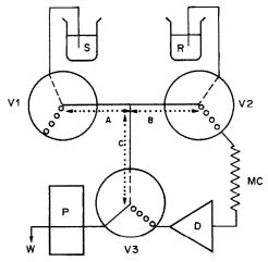
Fig. 1. Simplest ACCAS configuration. V1-3: 3-way valves; S: sample, R: reagent; MC: mixing coil, D: detector, P: pump, W: waste.
