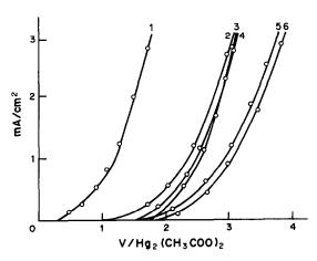
Fig. 3. Change of the anodic potential (vs. mercurous acetate reference) with current density in 0.25M solution of sodium perchlorate in acetic acid-acetic anhydride (1:6) mixture:
