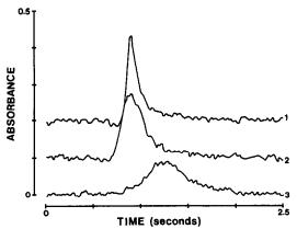
Fig. 3. Absorption profiles for 25  $\mu$ g/l. tin: 1, modifier A; 2, modifier B; 3, modifier C.
