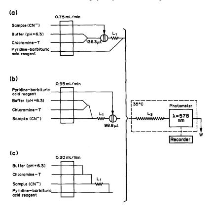
Fig. 7. Manifolds for determination of cyanide: (a) normal FIA; (b) reverse FIA; (c) completely continuous technique. 32
