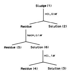
Fig. 1. Scheme for the fractionating procedure. Solution 2: HCl-soluble compounds (basic compounds, carbohydrates); solution 6: NaOH-soluble compounds (weak acids, fulvic and humic acids, complex polysaccharides); solution 3: NaOH-extractable and HCl-soluble compounds (e.g., fulvic acids); residue 4: NaOH-extractable and HCl-insoluble compounds (e.g., humic acids); residue 5: compounds insoluble in 0.1M HCl and 0.1M NaOH.
