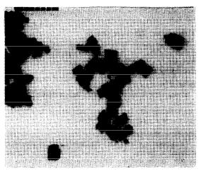
ig. 2. Electron micrograph of Na<sub>2</sub>Zn<sub>3</sub>[Fe(CN)<sub>6</sub>]<sub>2</sub>. Magnification, 3 × 10<sup>4</sup>.
