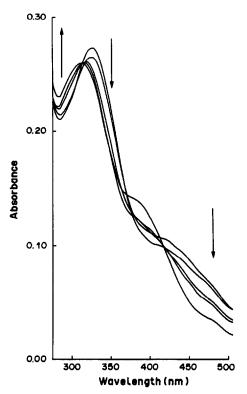
Fig. 3. Absorption spectra of the system Pd(II)-NMP at different pH values. Arrows indicate the spectral trends in changing the pH from 1.11 to 5.46.  $C_L = 2.70 \times 10^{-5} M$ ,  $C_M = 9.81 \times 10^{-6} M$ .
