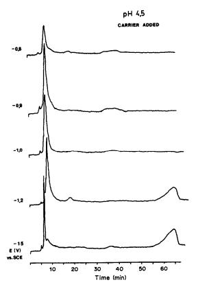
Fig. 7. HPLC of "carrier added" 99mTc-HEDP mixtures prepared by coulometric reduction of TcO<sub>4</sub> at pH 4.5 and various reduction potentials. Conditions as for Fig. 5.
