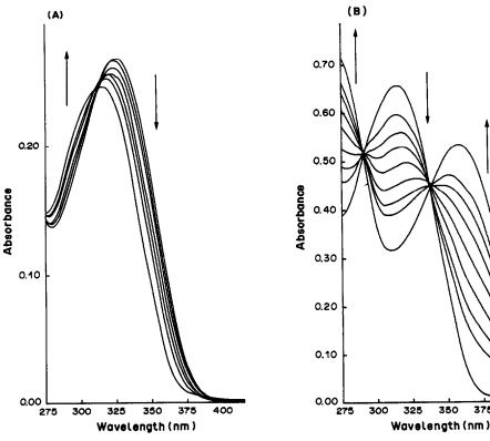
Fig. 1. Spectra of two series of solutions used to determine the protonation constants of H<sub>2</sub>NMP. Arrows indicate the spectral trends in changing the pH (A) from 1.11 to 5.72,  $C_L = 3.03 \times 10^{-5} M$ ; (B) from 5.66 to 11.74,  $C_L = 7.98 \times 10^{-5} M$ .
