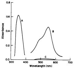
Fig. 1. Absorption spectra of (A)  $1.25 \times 10^{-4}M$  DCDT in DMF, (B) Fe(II)-DCDT complex at pH 0.36 [ligand  $5 \times 10^{-4} M$ , Fe(II)  $5 \times 10^{-5} M$ ], and (C) Fe(III)-DCDT complex at pH 0.36 [ligand  $5 \times 10^{-4}M$ , Fe(III)  $1 \times 10^{-4}M$ ].
