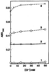
Fig. 4. Effect of CT concentration on extent of chloride interference. Curve (1) [CT] =  $38.6\mu M$ ; [Br] =  $0\mu M$ ; (2) [CT] =  $38.6\mu M$ ; [Br] =  $25\mu M$ ; (3) [CT] =  $386\mu M$ ; [Br] =  $0\mu M$ ; (4) [CT] =  $386\mu M$ ; [Br] =  $25\mu M$ .
