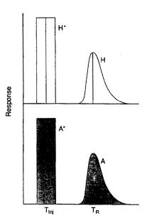
Fig. 4.  $D^{\text{max}}$  pictorially compared to  $X^{-1}$ . (A) peak height at steady state divided by height at peak maximum equals  $D^{\text{max}}$ . (B) Injected "area" (number of moles) divided by peak area equals  $X^{-1}$ .
