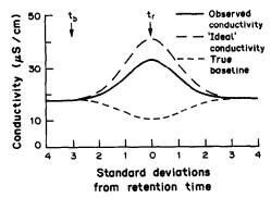
Fig. 4. Model peak for  $2.5 \,\mu$ mole of determinand with carbonate eluent. Notation as in Fig. 3.
