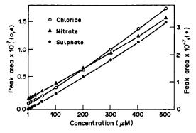
Fig. 1. Calibration graphs for chloride  $(\bigcirc)$ , nitrate  $(\triangle)$  and sulphate  $(\blacksquare)$ .
