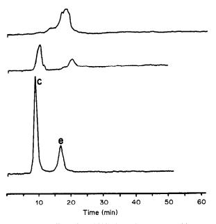
Fig. 11. The effect of an RVC electrode on the resulting 99mTc-HEDP mixture prepared by coulometric reduction at -1.000 V and pH 5.6.
