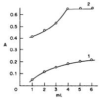
Fig. 2. Variation of the reaction rate with volume of reduced Rhodamine B solution. (1) Uncatalysed reaction;
