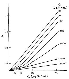
Fig. 6. Effect of aluminium on the calibration curve for strontium in the air-acetylene flame.
