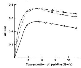
Fig. 4. Influence of pyridine concentrations on the colour intensity developed from: 1 μmole of penicillin G sodium (——); 2 μmole of ampicillin (....); 3 μmole of cephalexin sodium (-···-).
