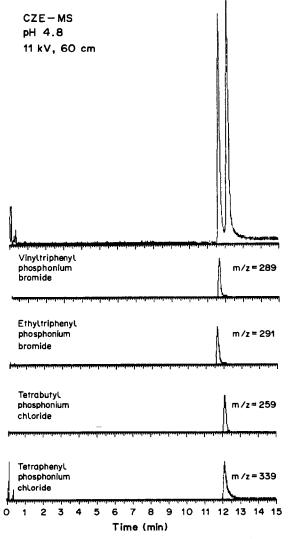
Fig. 9. Total and single-ion electropherograms for a CZE-MS separation of a mixture of quaternary phosphonium salts at pH 4.8 in a 60 cm  $\times$  100  $\mu$ m capillary at 11 kV.
