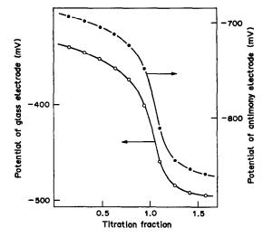
Fig. 6. Response of glass (○) and antimony/antimony oxide (●) electrodes in the titration of MEA + CO<sub>2</sub> reaction product in 2-propanol + water (98 + 2).
