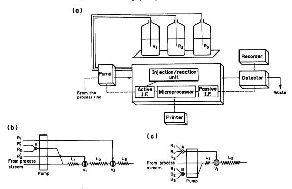
Fig. 11. Completely automated analyser for on-line control. (a) Block diagram. The assembly formed by the propelling, injection and reaction units can adopt configurations (b) and (c). R, reagent; L, reactor; V, injection valve, A and B, selecting valves.
