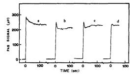
Fig. 4. Changes in photoacoustic signal amplitudes when a 506-nm laser beam was incident on Hg(II) dithizonate solutions in (a) CHCl<sub>3</sub>, (b) benzene, (c) benzene-CCl<sub>4</sub> and (d) benzene-CCl<sub>4</sub> (with 100-sample boxcar averaging).
