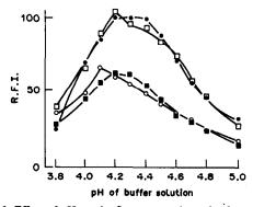
Fig. 3. Effect of pH on the fluorescence intensity for  $1.0 \mu g$  of caffeine. The buffers were prepared by mixing the buffer components to give the desired pH. Components:  $\bullet$ , 0.6M acetic acid-0.6M sodium acetate;  $\blacksquare$ , 0.6M citric acid-1.2M disodium hydrogen phosphate;  $\square$ , 0.6M hydrochloric acid-0.6M sodium acetate;  $\bigcirc$ , 0.6M citric acid-sodium citrate.
