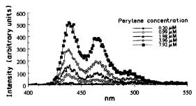
Fig. 3. Perylene TR emission spectra as a function of perylene concentration.
