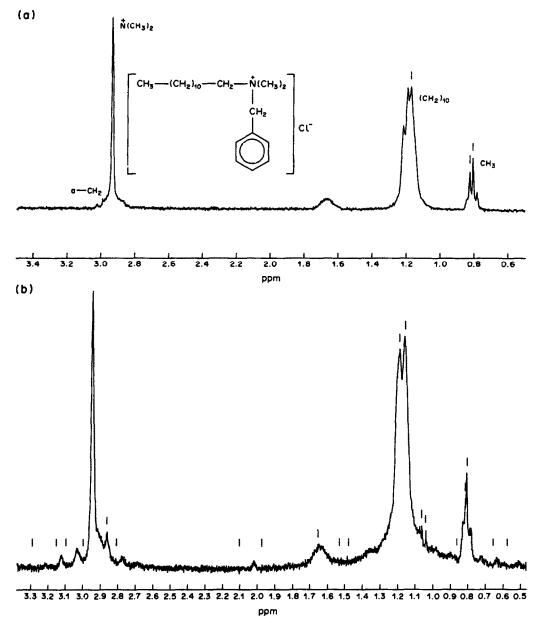
Fig. 1. Proton NMR spectra in  $D_2O$  of (a)  $1.0 \times 10^{-2}M$  BAC; (b)  $1.0 \times 10^{-2}M$  BAC saturated with anthracene.
