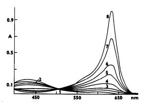
Fig. 2. Absorption spectra as a function of  $UO_2^{2+}$ -concentration in the calibration.  $c_L = 1 \times 10^{-5} M$ ,  $c_T = 8 \times 10^{-4} M$ , pH 5.6,  $I = 0.05 c_M$ ; 1, 0; 2, 0.25 ×  $10^{-6} M$ ; 3, 0.5 ×  $10^{-6} M$ ; 4,  $1 \times 10^{-6} M$ : 5,  $2 \times 10^{-6} M$ ; 6,  $3 \times 10^{-6} M$ ; 7,  $5 \times 10^{-6} M$ ; 8,  $7 \times 10^{-6} M$ .
