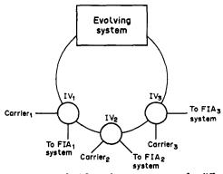
Fig. 10. Common feed from the process stream for different FIA manifolds. IV, injection valves.
