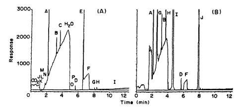
Fig. 12. Reconstructed chromatograms from the Cryofocus GC/FT-IR analysis of volatile components in the headspace of unprinted (A) and printed (B) cellophane package wrappers heated to 90° for 4 hr.
