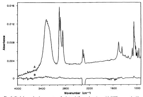
Fig. 8. Single-beam absorbance spectra of n-butanol (5 monolayers) on nickel(100) measured with p-polarized light (A) and s-polarized light (B).
