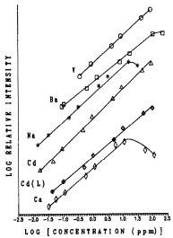
Fig. 5. Analytical calibration curves for each element.
