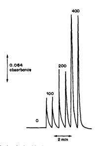
Fig. 1. Peaks obtained by injection of 0, 100, 200, 400 ppm standard solutions of caffeine: flow-rate 1 ml/min, injection volume 10  $\mu$ l.
