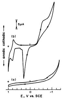
Fig. 1. Cyclic voltamperograms obtained with a carbonpaste electrode modified with TTCT: (a) in 0.1M acetate buffer (pH 4.5); (b) in 0.1M acetate buffer (pH 4.5) after accumulation for 1 min from 50μM Ag(I) in 0.1M sodium perchlorate. Scan-rate 50 mV/sec.
