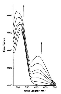
Fig. 2. Absorption spectra of the system Ni(II)-NMP at different pH values. Arrows indicate the spectral trends in changing the pH from 3.27 to 4.98.  $C_L = 7.04 \times 10^{-5} M$ ,  $C_M = 3.22 \times 10^{-5} M$ .
