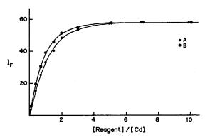
Fig. 3. Influence of the concentrations of cryptand 2.2.1 (A) and eosin (B) on fluorescence intensity:  $C_{\rm Cd} = 8.90 \times 10^{-7} M$ , (A)  $C_{\rm E} = 1.4 \times 10^{-5} M$ ,  $C_{\rm L}/C_{\rm Cd}$  varied. (B)  $C_{\rm L} = 1.4 \times 10^{-5} M$ ,  $C_{\rm E}/C_{\rm Cd}$  varied.  $I_{\rm F}$  in arbitrary units.
