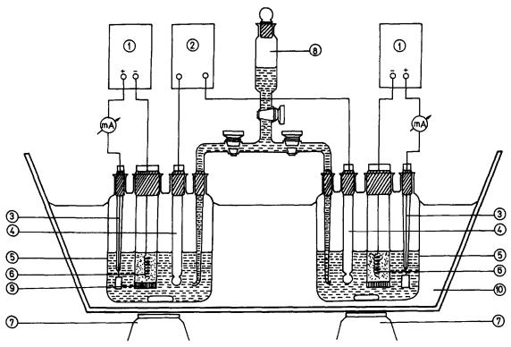
Fig. 1. Schematic diagram of the apparatus for the potentiometric determination of  $pK_A$  values of bases in anhydrous acetone with coulometrically generated protons: 1—current stabilizer, 2—pH-meter, 3—H<sub>2</sub>/Pd electrode, 4—glass electrode, 5—electrolytic vessel, 6—Pt cathode, 7—magnetic stirrer, 8—electrolytic bridge, 9—G-4 sintered-glass disc, 10—oil bath.
