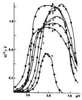
Fig. 4. Apparent molar absorptivity at 630 nm vs. pH plots for the system UO<sub>2</sub><sup>+</sup>-CAB-Septonex for solutions with varied concentrations of components.  $c_{\rm M}=7\times10^{-6}M$ ,  $c_{\rm T}=\times10^{-3}M$ .  $c_{\rm L}/c_{\rm M}$ : curve 1, 1.0; curve 2, 2.0 curve 3, 3.5; curve 4, 5.0; curve 5, 10.0; curve 6,  $c_{\rm L}=7\times10^{-6}M$ ,  $c_{\rm M}/c_{\rm L}=149$ ,  $c_{\rm T}=1\times10^{-3}M$ ; curve 7,  $c_{\rm L}/c_{\rm M}=2$ ,  $o_{\rm T}=1.5\times10^{-2}M$ .
