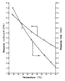
Fig. 18. The signal response and response time vs. temperature curves obtained with interface B (Fig. 15) for p-limonene in air.
