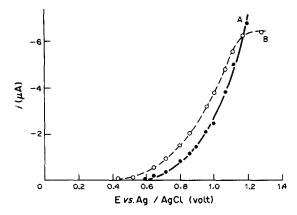
Fig. 2. Voltamperogram showing the response to pure NO(g) at a polymer-coated glassy carbon electrode (A) and a modified carbon paste electrode (B). Carrier supporting electrolyte 0.10M KCl (pH 4.00). Flow-rate 2.0 ml/min. Injected sample size 250 μl.
