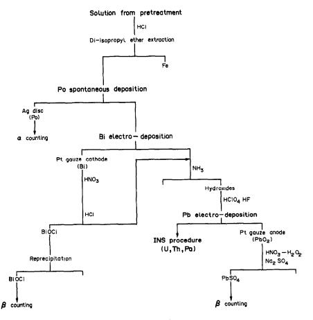
Fig. 1. Schematic diagram of the analytical procedure.
