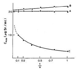
Fig. 7. Determination of strontium in the presence of vanadium in the air-acetylene flame. Test sample:  $20~\mu g$  Sr/ml and 1 mg V/ml. Curve A: without buffer interferent;  $c_{App_{\infty}} = 20.2~\mu g$ /ml. Curve B: buffer interferent 5 mg Al/ml;  $c_{App_{\infty}} = 21.3~\mu g$ /ml. Curve C: evaluation by Gilbert's dilution method;  $c_{App_{\infty}} = ?$
