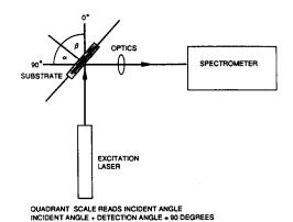
Fig. 2. Experimental set-up for angle of incidence studies  $(\alpha = \text{detection angle}; \beta = \text{incidence angle}).$
