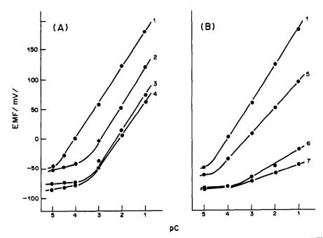
Fig. 2. Calibration curves of cloxacillin electrode. A: 1—cloxacillin; 2—benzylpenicillin; 3—ampicillin; 4—amoxycillin; B: 1—cloxacillin; 5—nitrate; 6—chloride; 7—acetate.
