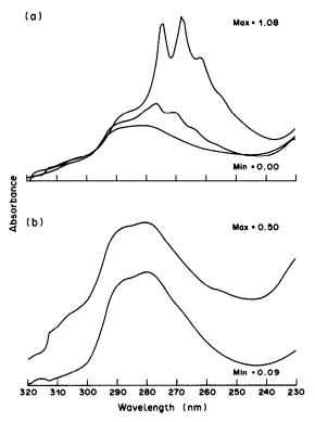
Fig. 5. (a) Spectra of an n-heptane extract of a Berthelot reaction mixture (upper spectrum) and the same n-heptane phase after two successive washes with an equal volume of water (lower two spectra). (b) Comparison of the spectrum of chlorimine in n-heptane (lower curve) with the spectrum obtained by extracting and isolating an intermediate from an aqueous solution undergoing the Bertholet reaction. The solutions are not of equal concentration.
