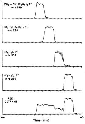
Fig. 12. Capillary isotachophoresis-MS separation of the quaternary phosphonium salt mixture in a 2 m  $\times$  100  $\mu$ m i.d. capillary at 35 kV.
