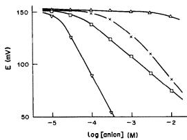
Fig. 4. Potentiometric response of a typical TFABB-doped hydroxylated asymmetric membrane to various anions in a background of 0.1*M* Tris-H<sub>2</sub>SO<sub>4</sub>, pH 8.75: (△) Cl<sup>-</sup>; (×) NO<sub>5</sub>; (□) total CO<sub>2</sub> (predominantly carbonate and hydrogen carbonate); (▽) salicylate.
