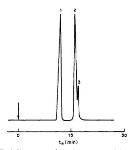
Fig. 8. Chromatogram of n-butyl acetate extract of phenol and cresols from aqueous solution: (1) o-cresol, (2) m- and p-cresol, (3) phenol. Column Silasorb 600, 10  $\mu$ m, 200  $\times$  6 mm; mobile phase 15% v/v chloroform in n-heptane; 25°C; Spectrophotometric detector (270 nm).
