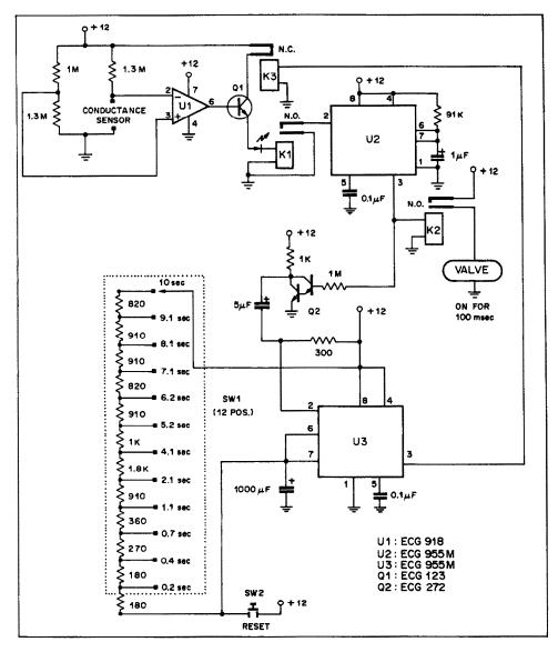
Fig. 7. Schematic of circuitry used for automated pulsed reagent-introduction.
