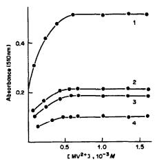
Fig. 3. Dependence of Fe(II)(phen), yield on initial concentration of methylviologen. [EDTA] = 0.02M, other conditions as for Fig. 2: (1) proflavine and acriflavine, (2) Acridine Orange, (3) Acridine Yellow, (4) rivanol.
