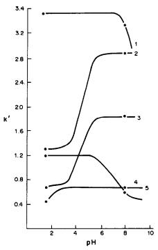
Fig. 1. A plot of capacity factor against pH of mobile phase: 1—uridine; 2—cytosine arabinoside; 3—cytidine; 4—6-aza-uridine; 5—6-azacytidine.
