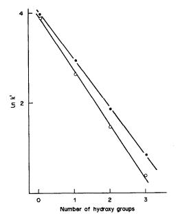
Fig. 3. Plots of ln k'vs. number of hydroxy groups on an aromatic ring. ●: data obtained before thermal treatment.
