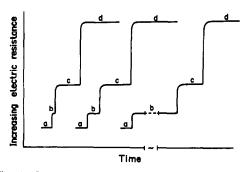
Fig. 1. Graphical representation of isotachophorograms obtained for the extracts from the surfaces of differently heated porous glasses: (a) electric resistance of leading electrolyte, (b) electric resistance of BO<sub>2</sub><sup>-</sup> zone, (c) electric resistance of SiO<sub>3</sub><sup>2</sup> - zone, (d) electric resistance of terminal electrolyte. Lengths of segments are proportional to concentration of the species concerned.
