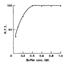
Fig. 4. Effect of acetic acid-sodium acetate buffer concentration (pH 4.3).
